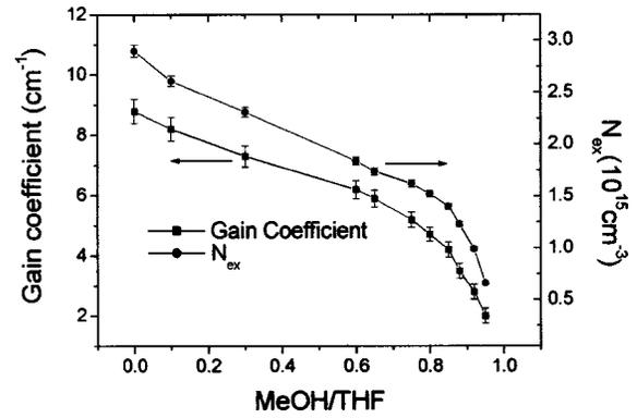
FIG. 3. The gain coefficient  $g$  and the excited isolated chains concentration  $N_{\text{ex}}$  as a function of MeOH/THF. Both exhibit a gradual decrease becoming more intense for MeOH/THF > 0.65.
