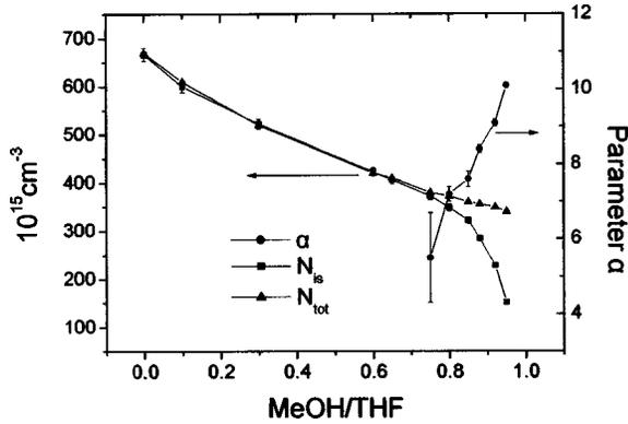
FIG. 4. The isolated chains concentration  $N_{is}$  and the total polymer concentration  $N_{tot}$  as a function of MeOH/THF. For MeOH/THF > 0.65, the two curves are separated indicating the formation of aggregates. For these solutions the parameter  $\alpha$  is also plotted.
