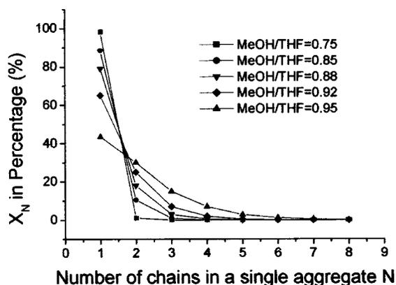
FIG. 5. The distribution of polymer chains  $X_N$  in percentage as a function of the aggregation number  $N$  for values of MeOH/THF  $> 0.65$ , where aggregates are formed.
