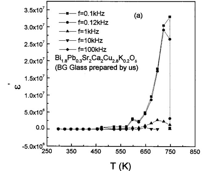
FIG. 2. Variation of the real part of dielectric constant  $\epsilon'$  vs  $T$  of (a) our BG glass viz.  $\text{Bi}_{1.8}\text{Pb}_{0.3}\text{Sr}_2\text{Ca}_2\text{Cu}_{2.8}\text{K}_{0.2}\text{O}_8$  and (b) a typical MP glass viz.  $\text{Bi}_{3.9}\text{Pb}_{0.1}\text{Sr}_3\text{Ca}_3\text{Cu}_4\text{O}_x$  for different frequencies.
