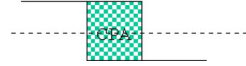
FIG. 4. (Color online) Two separate interfaces are used when studying interface scattering for free electrons. The first interface is a double potential step that has an intermediate potential level at the interface equal to the average of the two bulk potentials. In the LKKR calculation, this potential region is approximated as a CPA alloy layer.
