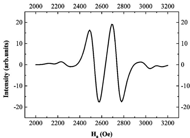
FIG. 6. Computer simulation of the ESR signal for  $\phi=0^\circ$  with hyperfine structure included both for <sup>171</sup>Yb and <sup>173</sup>Yb isotopes. The linewidth was set to 60 Oe.
