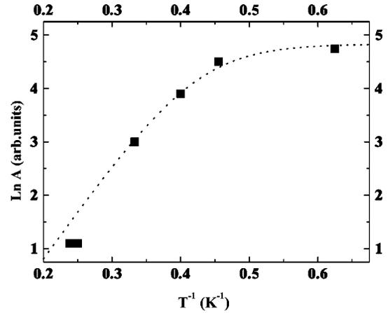
FIG. 5. Temperature dependence of the maximum-to-minimum amplitude of the ESR line for  $\phi = 90^\circ$ . Dotted curve is drawn according to the relation  $D/[1 + R \exp(-\Delta/T)]$  with  $D = 125$ ,  $R = 2000$ , and  $\Delta = 18$  K.
