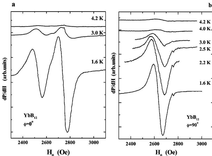
FIG. 2. a. ESR spectra for several temperatures in the 1.6–4.2 K range at  $\phi=0^\circ$ . b. ESR spectra for several temperatures in the 1.6–4.2 K range at  $\phi=90^\circ$ .
