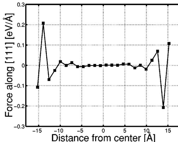
FIG. 1. Force on the atoms, along the [111], due to the presence of a domain boundary. The forces are plotted as a function of distance from the center of the unit cell. The domain boundary is generated such that the nearest-neighbor distance is always within 95% of the bulk ( $\alpha = 1/4$ ).
