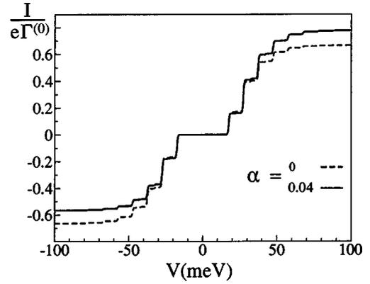
FIG. 6.  $I$ - $V$  characteristics with  $c_2=0$ ,  $c_1=1.5$ ,  $\alpha=0, 0.04$ , and  $E_c=20$  meV.
