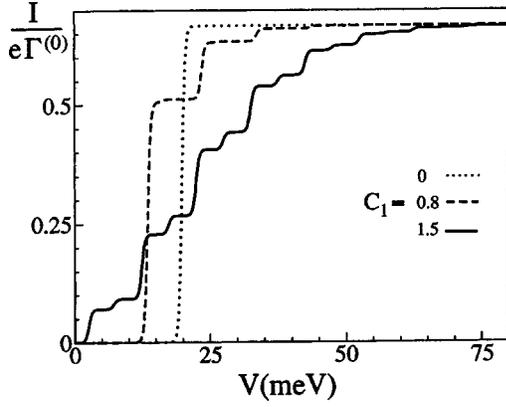
FIG. 2.  $I$ - $V$  characteristics for  $c_2=0$ ,  $c_1=0.0, 0.8, 1.5$  with the voltage offset for each curve defined by the parameter  $E_c = 10$  meV (see text).
