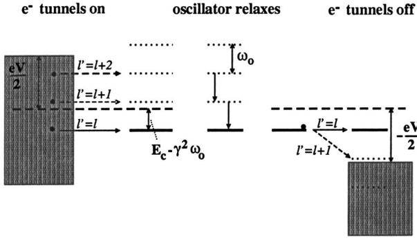
FIG. 1. Schematic of  $C_{60}$  transistor system in terms of combined electronic-vibrational transitions for passage of current through the device. Dashed arrows indicate transitions in which quanta of oscillator energy  $\hbar\omega_0$  are supplied to the  $C_{60}$  by the tunneling electron.
