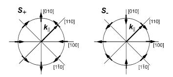
FIG. 2. Spin orientation of eigen states "+" and "-" as a function of the orientation of the in-plane electron wave vector  $k_{\parallel}$ .
