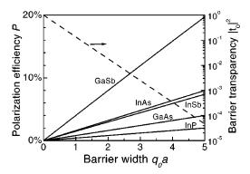
FIG. 3. Coefficient of the polarization efficiency  $\mathcal{P}$  as a function of barrier width  $aq_0$  for various barrier materials, and  $k_{\parallel}=2 \times 10^6$  cm<sup>-1</sup>. Dashed line presents the barrier transparency.
