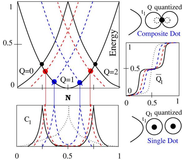
FIG. 2. Charging energies ( $+\delta E$ ) of the “composite” dot as a function of  $N$  given in units of  $E_c$ ;  $t_1$  is small. Each eigenstate with  $Q=n$  gives rise to a parabola. The solid lines correspond to  $r_2=0$  and dashed lines to increasing  $r_2$  couplings. For  $r_1=1-t_1 \rightarrow 1$ ,  $Q$  is quantized and for symmetric dots this guarantees  $\bar{Q}_1 = n/2$  until  $r_2 \rightarrow 1$  [Eqs. (11) and (24)].
