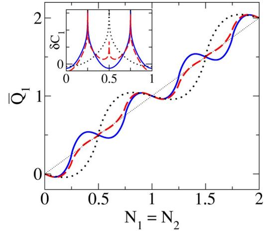
FIG. 4. Evolution of the fractional plateaus for *small*  $r_1$ . [Note, e.g., that for  $r_2=0$  we have only taken into account the main leading term when taking the derivate of Eq. (19), which explains the “slightly” negative slope in the middle of a plateau]. The solid line is for  $r_1=0.2$  and  $r_2=0$ , the dashed line for  $r_1=r_2=0.15$  (fractional plateaus now acquire a *positive* slope) and the dotted line for  $r_1=0.3$  and  $r_2 \rightarrow 1$ .
