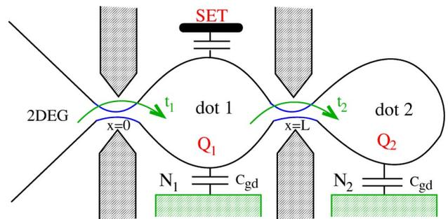
FIG. 1. A two-dimensional electron gas (2DEG) is coupled to two *large* dots via a single-mode QPC. The number of electrons  $Q_i$  on each dot is controlled via the dimensionless gate voltage  $N_i$ . The case of interest here is  $N_1 = N_2 = N$ . The auxiliary gates can be used to adjust the conductances at the QPC’s. A SET may probe the average charge on a single dot.
