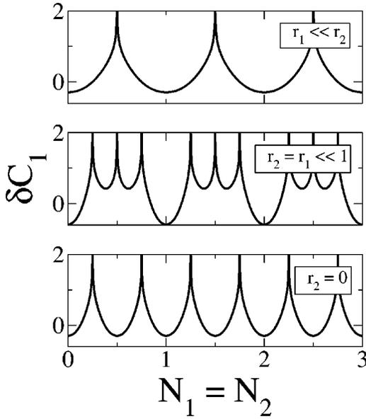
FIG. 3. Dot's differential capacitance for *small*  $r_1=0.4$ . For  $r_2 \approx 0$  the system behaves as a single *composite conductor* whereas for  $r_2 \rightarrow 1$  we must recover a *single-dot* problem. For  $r_2 \approx r_1 \ll 1$  the system cannot decide between those two ground states giving a “three-peak” capacitance profile, i.e., unstable fractional steps [Fig. 4 and Eq. (22)]. Charge fluctuations are important at  $N=1/4$  and at  $N=1/2$  as well.
