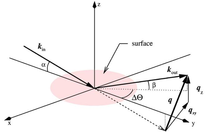
FIG. 2. Kinematics of the x-ray measurement.
