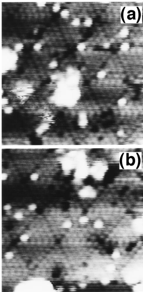
FIG. 4. STM images (a) before and (b) after FE irradiation (50 eV) to Si(111)- $7\times 7$  surfaces dosed with 50 L of Br<sub>2</sub> at 400 °C. (a) was taken at a sample bias of +2.0 V and a tunneling current of 0.8 nA. (b) was taken at a sample bias of +1.0 V and a tunneling current of 0.8 nA. The areas shown are  $7.8\times 7.8$  nm.
