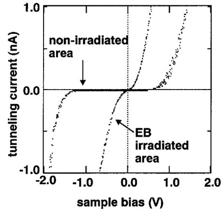
FIG. 2. Tunneling current-sample bias ( $I$ - $V$ ) curves measured over nonirradiated and FE-irradiated areas of the sample surface shown in Fig. 1(a). The feedback loop was inactivated at a sample bias of +1.0 V and a tunneling current of 0.7 nA.
