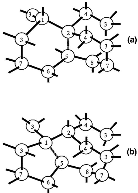
FIG. 5. Three-dimensional illustration of (a) the ideal Si(111) surface and (b) the Si(111)- $2\times 1$   $\pi$ -bonded chain reconstruction.
