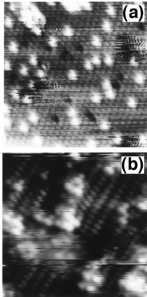
FIG. 3. STM images (a) before and (b) after Fe irradiation (50 eV) to Si(111)- $7\times 7$  surfaces dosed with 100 L of  $\text{Br}_2$  at  $450^\circ\text{C}$ . (a) was taken at a sample bias of +2.0 V and a tunneling current of 0.8 nA. (b) was taken at a sample bias of +1.0 V and a tunneling current of 0.8 nA. The areas shown are  $7.8\times 7.8$  nm.
