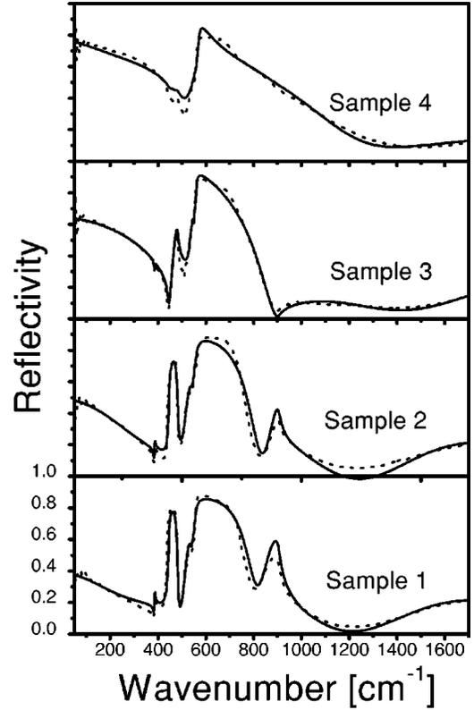
FIG. 1. IR reflection spectra of GaN epilayers on sapphire substrate. Dotted lines, experimental; solid lines, theoretical fitting spectra.
