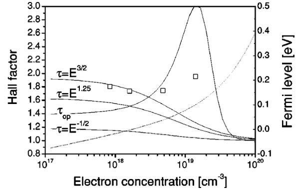
FIG. 2. Hall factors of individual scattering processes as functions of the carrier concentration in the GaN epilayer at room temperature. The dotted line is the Fermi level.  $\square$ 's are measurement data.
