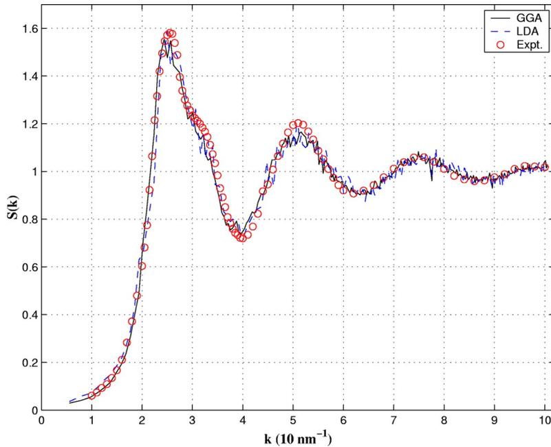
FIG. 1. (Color online) Static structure factor  $S(k)$  for  $l$ -Ge at  $T=1250$  K, just above the experimental melting temperature. Full curve: present work, as calculated using the generalized gradient approximation (GGA; see text). Dashed curve: present work, but using the local-density approximation (LDA; see text). Open circles: measured  $S(k)$  near  $T=1250$  K, as given in Ref. 34.
