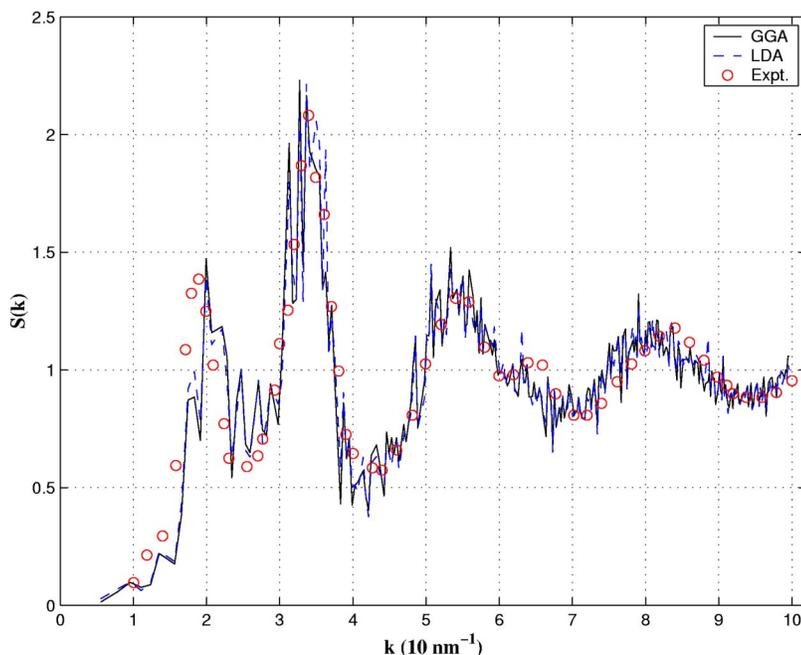
FIG. 2. (Color online) Full curve: Calculated  $S(k)$  for  $a$ -Ge at  $T=300$  K, as obtained using the GGA. Structure is prepared as described in the text. Dashed curve: same as full curve, but calculated in the LDA. Open circles: measured  $S(k)$  for  $a$ -Ge at  $T=300$  K, as given in Ref. 35.
