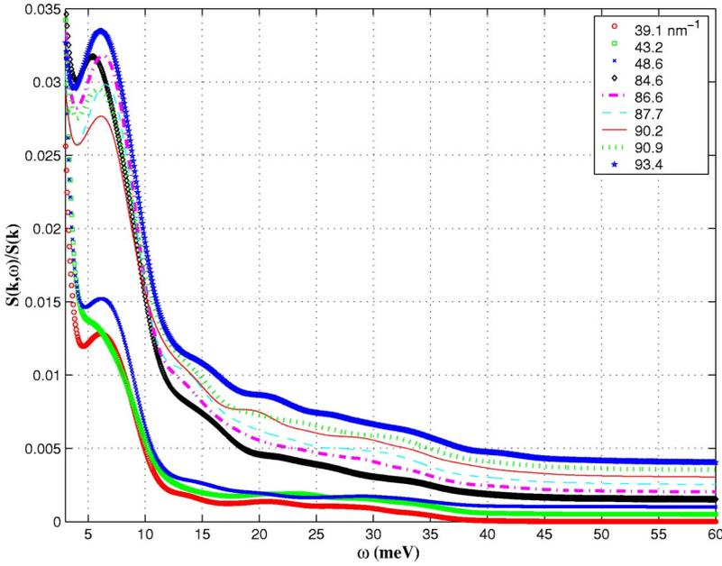
FIG. 7. (Color online) Calculated  $S(k, \omega)/S(k)$  as in Figs. 5 and 6 but including higher frequencies  $\omega$ . At  $\hbar\omega = 60$  meV, the curves are arranged vertically in order of increasing frequency. Each curve is vertically displaced by 0.0005 units from the one below it.
