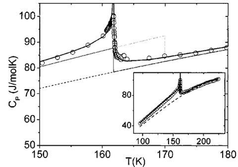
FIG. 3.  $C_p$  data (open circles), polynomial background  $C_{\text{poly}}$  (dashed line). Dotted line: calculated  $C_{\text{MF}}$  that conserves entropy, truncated above  $T_c$  to give a mean-field contribution to fit (thin line). Thick line: fit to  $C_p$  including Gaussian fluctuations. Inset:  $C_p$  data, fit, and  $C_{\text{poly}}$  in wider temperature range.
