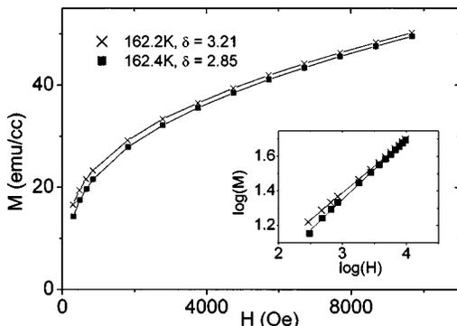
FIG. 2.  $M$  vs  $H$  at  $162.2$  and  $162.4$  K, closest to  $T_c = 162.26$  K. Inset:  $\log(M)$  vs  $\log(H)$ .
