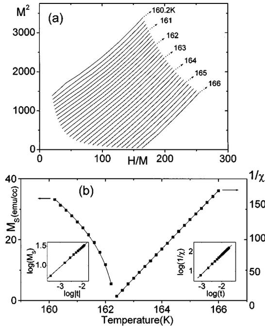
FIG. 1. (a)  $M^2$  vs  $H/M$  for single crystal  $\text{SrRuO}_3$  from  $T = 160$  to  $166$  K in  $0.2$ -K steps. (b)  $M_S$  and  $1/\chi$  [from intercepts in (a)] vs  $T$ . Insets: log-log plots for  $M_S$  and  $1/\chi$  vs reduced temperature  $t$ .
