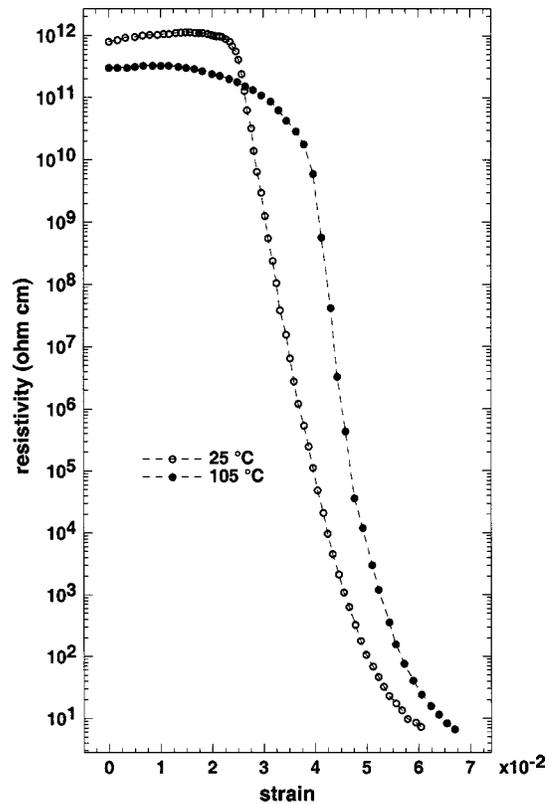
FIG. 5. The piezoresistance data of Fig. 4 nearly form a master curve when plotted against strain.
