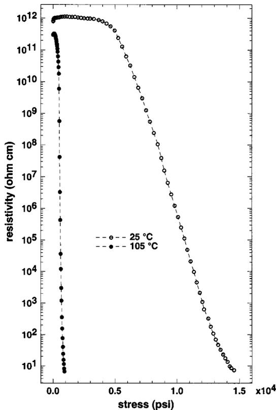
FIG. 4. Piezoresistance of an FSC of Au-coated Ni particles in epoxy. At 25 °C the epoxy is glassy, but at 105 °C it is rubbery and requires much less stress to deform.
