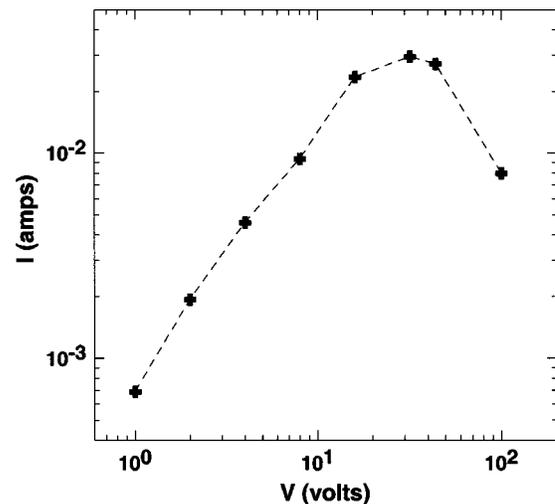
FIG. 8. The steady-state currents from the sample used to make Fig. 7 show an Ohmic regime followed by current-limiting behavior. The effect is reversible.
