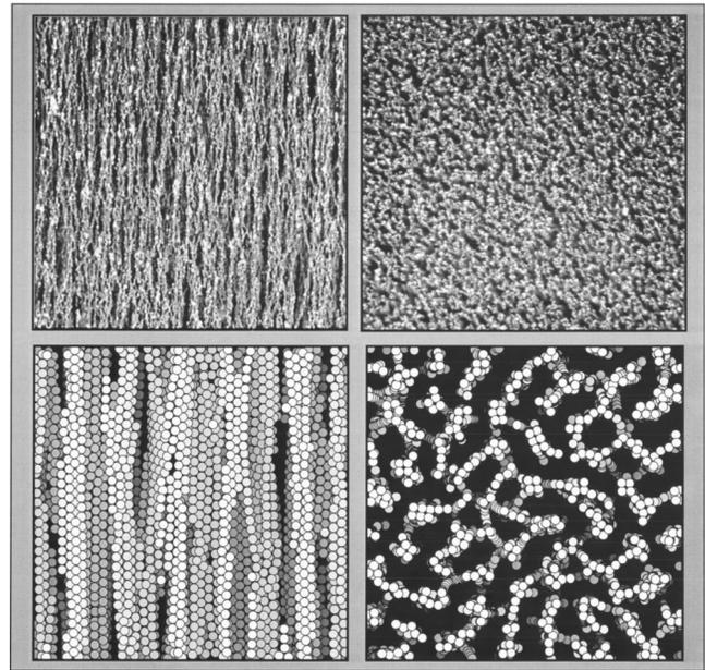
FIG. 1. Uniaxial FSC viewed perpendicular (top left) and parallel (top right) to the field structuring axis. Simulated uniaxial FSC viewed perpendicular (bottom left) and parallel (bottom right) to the field structuring axis. Particle volume fraction is 10.0%.
