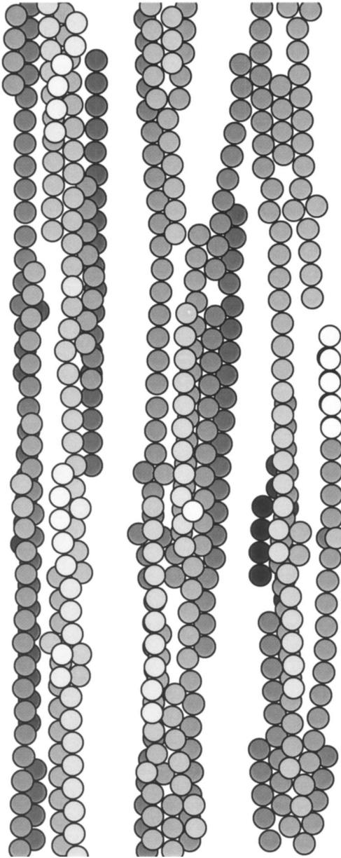
FIG. 9. Fragment of a large-scale simulation shows highly defective columns that bridge, forming cross links between chains.
