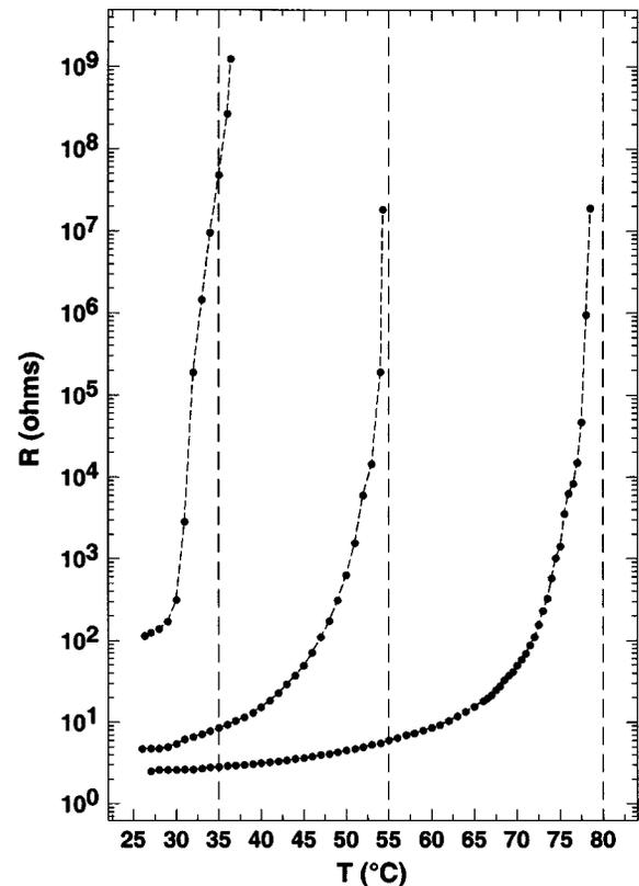
FIG. 3. Thermoresistance measurements of an FSC of Au-coated Ni particles in silicone show a conductivity divergence at, or close to, the cure temperature, each of which is indicated by a vertical dashed line.
