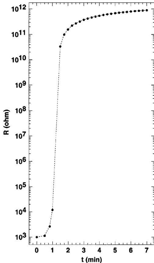
FIG. 6. Chemiresistance of an FSC of Au-coated Ni particles in silicone subjected to saturated toluene vapors (100 torr).
