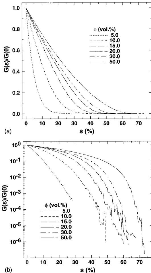
FIG. 11. (a) Conductivity of site percolation simulations on uniaxial FSC's of a wide range of concentrations show that at low concentrations, where chains are dominant, rendering only a small percentage  $s$  of particles nonconducting rapidly decreases the conductivity. (b) Plotting the data logarithmically shows a crossover from exponential behavior at low particle concentration to faster-than-exponential decay at higher concentrations.
