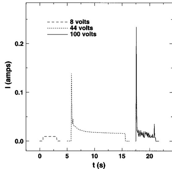
FIG. 7. When a potential is suddenly applied to a 1-cm-thick FSC of Au-coated Ni particles in epoxy resin, current limiting behavior can occur. The 8-V response is Ohmic, the 44-V response shows an initial current spike followed by current limiting behavior, and at 100 V the limiting current becomes extremely noisy.
