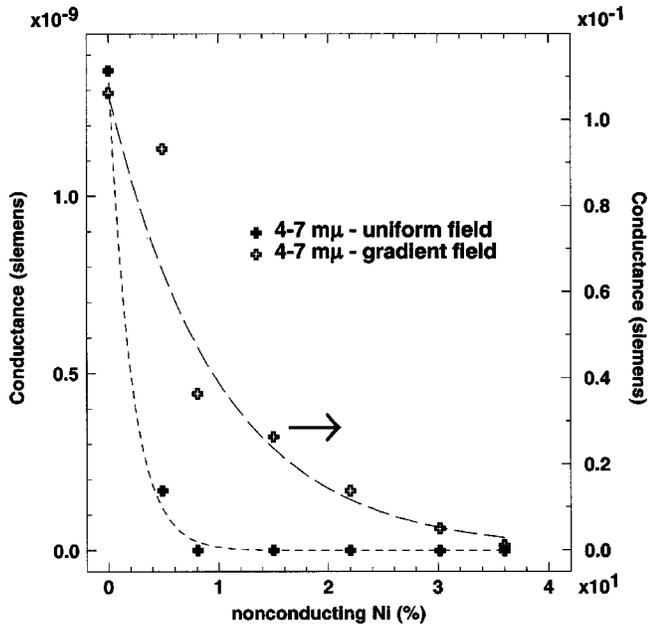
FIG. 10. Site percolation experiments on FSC's show an extremely rapid drop in sample conductance with the addition of nonconducting particles. The same particle suspensions show extremely large conductance when structured into dense powders using magnetic-field gradients.
