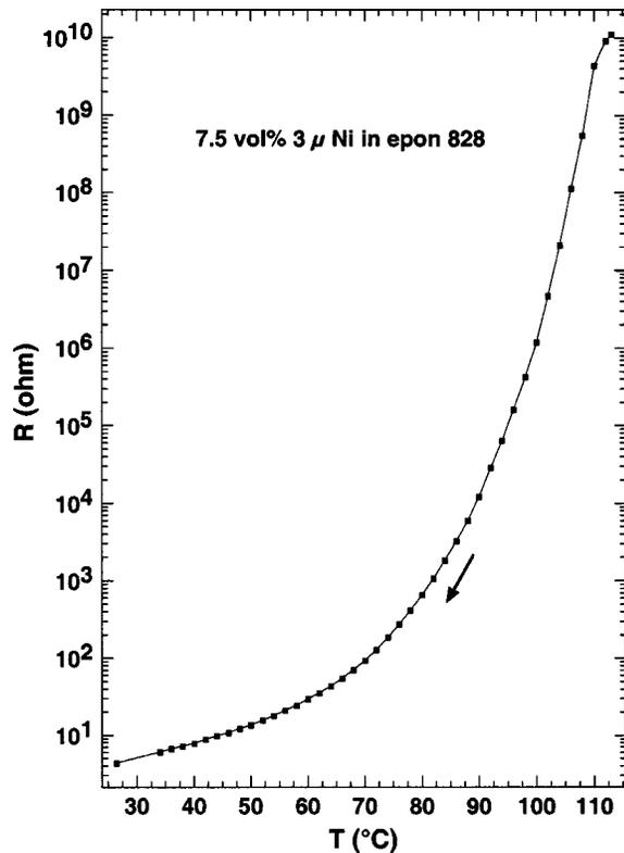
FIG. 2. Thermoresistance of an FSC of Au-coated Ni particles in epoxy. These data are taken below the glass transition temperature.
