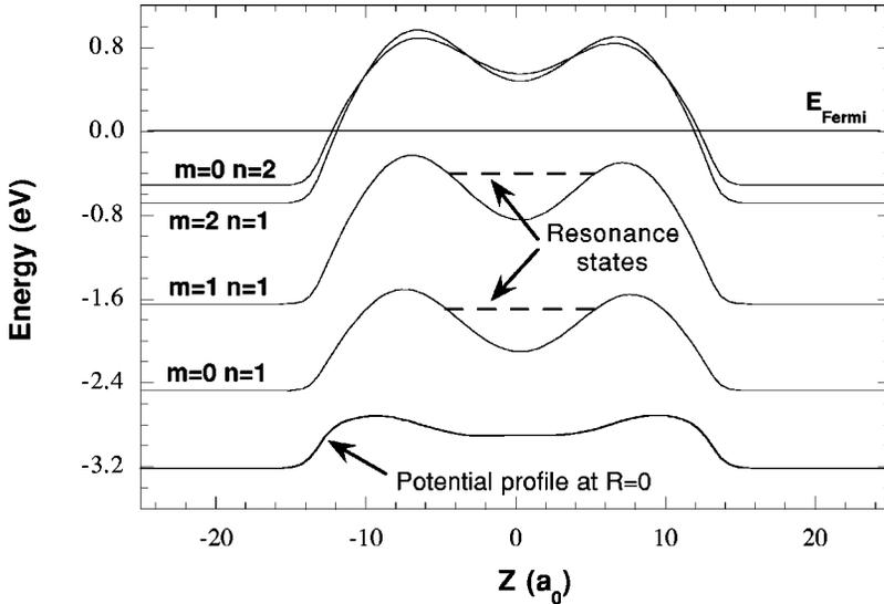
FIG. 8. Effective  $z$ -dependent potentials for the different  $(m, n)$  channels. The wire has eight UJ electrons and the elongation of  $\Delta L = 19.8a_0$  [Figs. 4(b) and 6]. The dashed lines in the potential wells are drawn at the energies of the resonance states. The lowest line is the bare Kohn-Sham potential at  $R=0$ .
