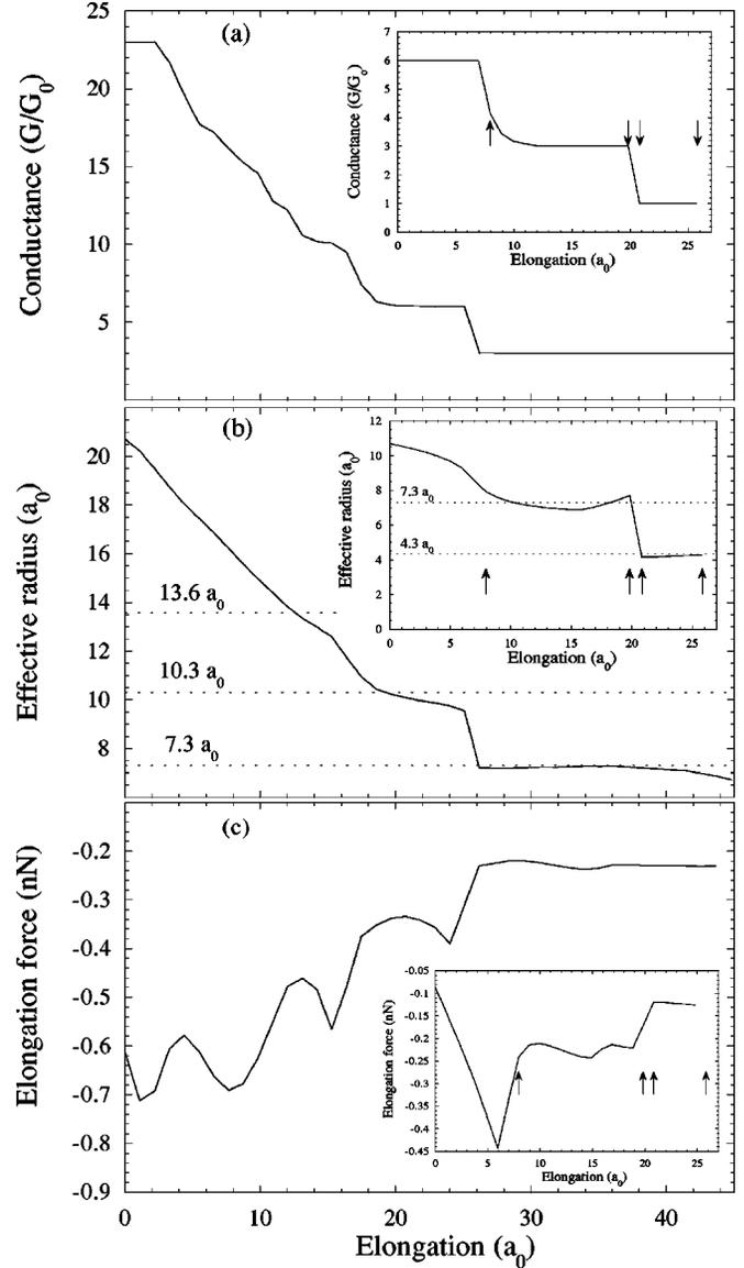
FIG. 5. Main figures: conductance, effective radius at the constriction, and elongation force for a wire with initial radius  $R = 20.7a_0$  and about 60 UJ electrons in the constriction. Insets: the same quantities for the wire in Fig. 4 with initial radius  $R = 10a_0$  and eight UJ electrons in the constriction. The arrows mark the points where the density has been plotted in Fig. 4.
