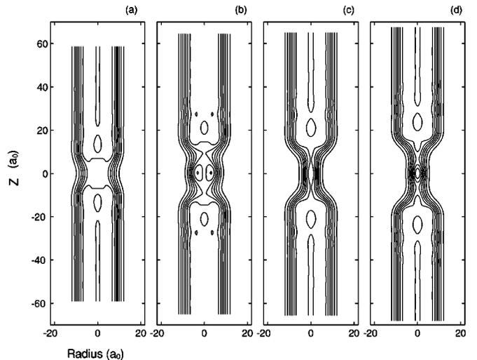
FIG. 4. Supported UJ wire. The UJ constriction contains eight electrons. Density contour plots for four different elongation lengths:  $\Delta L = 7.9a_0$  (a),  $19.8a_0$  (b),  $20.8a_0$  (c), and  $25.8a_0$  (d) are shown. The snapshots in (b) and (c) are from consecutive self-consistent calculations and the snapshot (d) is the last step before the nanowire breaking. The contour spacing is 0.15 times the mean UJ bulk density value.
