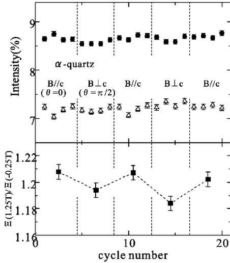
FIG. 2. Top: relative intensity of the positronium peak in  $\alpha$  quartz for two different orientations with regard to the magnetic field. (Closed circles: 1.25 T, open triangles:  $-0.25$  T.) Bottom: the ratio of the intensity of the positronium peak in the magnetic field of 1.25 T to that in  $-0.25$  T. The values are averaged over four scans in each orientation.
