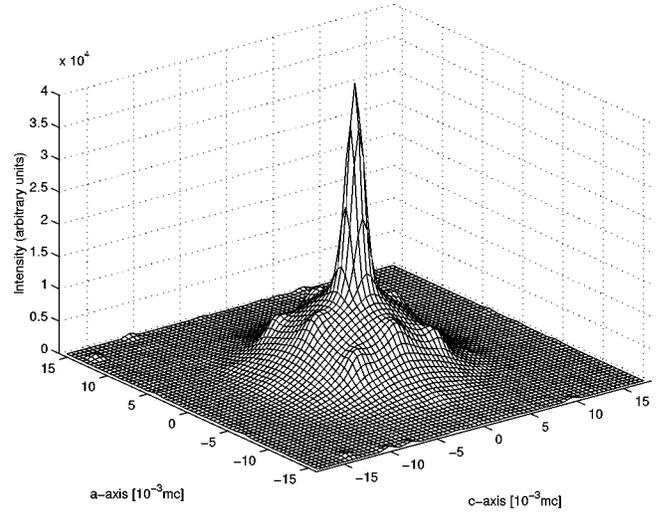
FIG. 1. 2D-ACAR spectrum for  $\alpha$  quartz.
