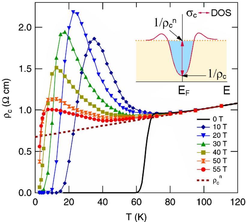
FIG. 2. (Color online)  $c$ -axis resistivity vs temperature in overdoped BSCCO up to 55 T. The normal ungapped state resistivity  $\rho_c^n(T)$  (dashed line) is evaluated from the measured  $T$ -linear dependence (Ref. 20) above  $T^*$  ( $\sim 100$  K). Inset:  $\rho_c$  corresponds to the inverse of the interlayer tunneling (differential) conductivity  $\sigma_c$  near Fermi energy  $E = E_F$ .
