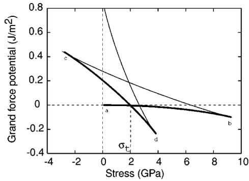
FIG. 2. Grand-force potential  $\phi$  for the traction curve of Fig. 1(a). Bold portions of the curves denote thermodynamically stable states.
