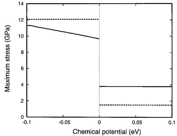
FIG. 3. Critical stress as a function of chemical potential relative to  $\mu_c$  (arbitrarily set to zero). Solid line is for hydrogen and dashed line is for oxygen.
