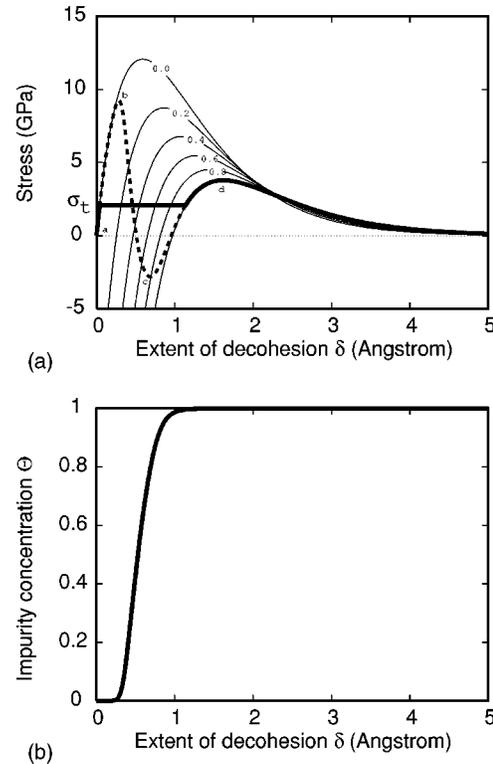
FIG. 1. (a) Traction curves calculated at different hydrogen concentrations  $\theta$  (thin lines).  $\theta$  is indicated along the traction curve. Superimposed is the traction curve at constant  $\mu$  (thick dashed line) greater than  $\mu_c$ . The thick solid line corresponds to the part of the traction curve with minimal grand-force potential. (b) Variation of  $\theta$  with slab separation  $\delta$  for a constant chemical potential above  $\mu_c$ .
