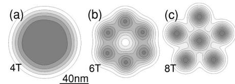
FIG. 2. Electron density distribution for six electrons in (a) approximation of the MDD phase for  $B=4$  T calculated with the six-center wave function in 1-5 configuration and the Wigner molecules with shell structures (b) 0-6 for  $B=6$  T and (c) 1-5 for  $B=8$  T. The darker the shade of grey the larger electron density. The bar shows the length scale.
