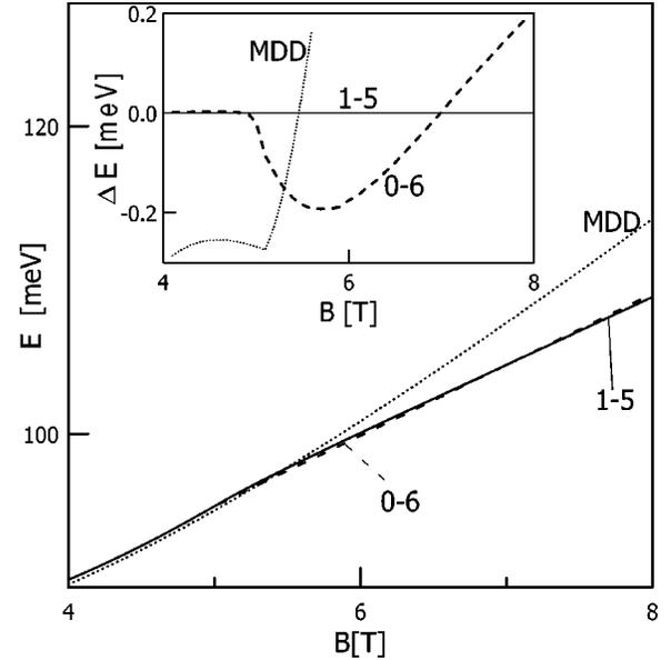
FIG. 1. Ground-state energy  $E$  of the six-electron Wigner molecule with shell-structure 1-5 (solid line) and 0-6 (dashed line), and the MDD phase (dotted line) as a function of magnetic field  $B$ . Inset shows the energy  $\Delta E$  of the 0-6 Wigner molecule and MDD determined with respect to the energy of the 1-5 (high-field) phase.
