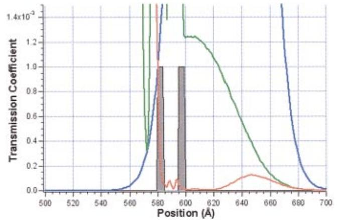
FIG. 4. (Color) A snapshot of the of the wave-function intensities shortly after the off-resonance wave packet (red) exits the tunneling structure. Note the presence of a small “echo” in the off-resonance transmission emphasizing that the transmission of this part of the wave packet is a transient effect. The leading edge of the off-resonance peak is slightly ahead of the on-resonance peak (green), but is lagging the leading edge of the unscattered freely propagating, wave packet (blue).
