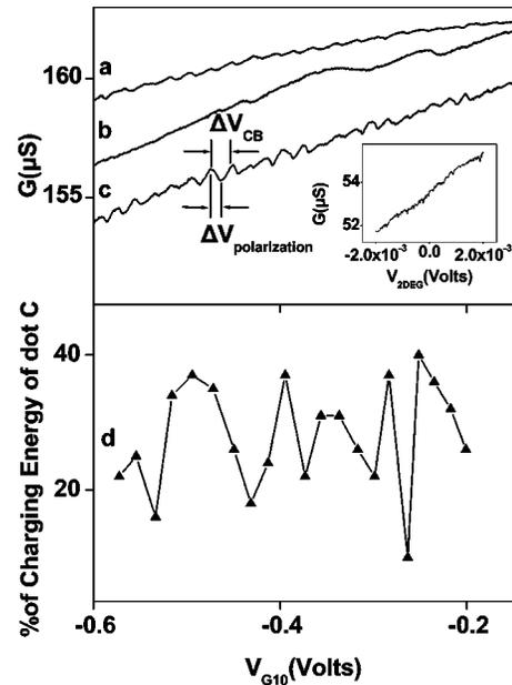
FIG. 2. Detector signal obtained (a) from dot C, (b) from dot D, (c) from the coupled dot pair of C and D. (d) The energy required to move one electron from dot C into dot D expressed as a percentage of the charging energy of dot C. The 1D ballistic channel between gates  $G_4$  and  $G_6$  was used as detector. In all cases, gate  $G_{10}$  was swept. Inset: Calibration of conductance into a voltage figure.
