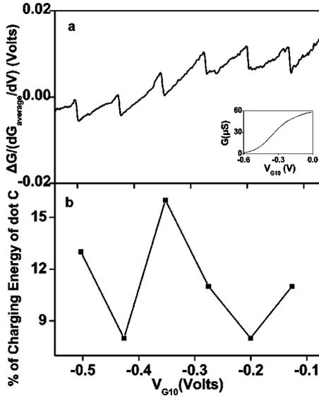
FIG. 3. (a) Detector signal obtained from the double-dot system of dots *C* and *D* when isolated from the reservoirs. (b) The energy required to move one electron from dot *C* into dot *D* expressed as a percentage of the charging energy of dot *C*.
