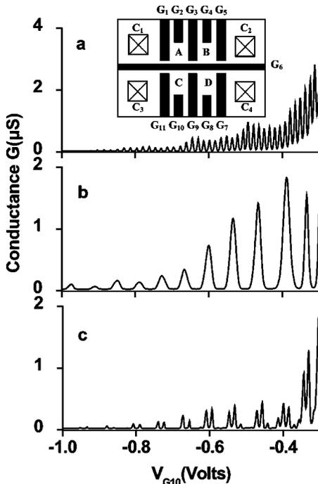
FIG. 1. Coulomb blockade oscillations of (a) dot C, (b) of dot D, and (c) of the coupled dot pair of C and D. In all cases the plunger of dot C,  $G_{10}$ , was swept. Inset: Schematics of the QCA cell.
