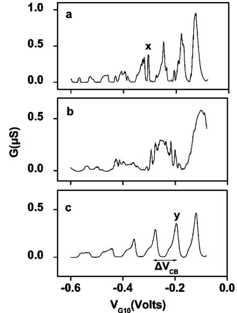
FIG. 4. Detector signal obtained from the coupled pair of dots *C* and *D* when (a) dot *B* was defined as detector, (b) the coupled pair of dots *A* and *B* was defined as detector. (c) Coulomb blockade oscillations of dot *B* when none of the dots *C* and *D* are defined. In all cases gate *G*10 was swept.
