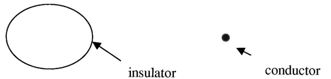
FIG. 10. An illustration of the structure of cellular composites. The small conducting particles are embedded on and between the surfaces of the larger insulator particles.
