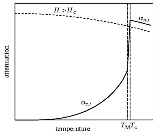
FIG. 1. Typical shear wave attenuation for a conventional superconductor with transition temperature  $T_c$ . The attenuation in the superconducting state  $\alpha_{s,t}$  drops rapidly with temperature until the Meissner effect is complete at  $T_M$ , then shows BCS behavior. The dashed curve shows the effect on the normal state attenuation  $\alpha_{n,t}$  of a magnetic field larger than the critical field.
