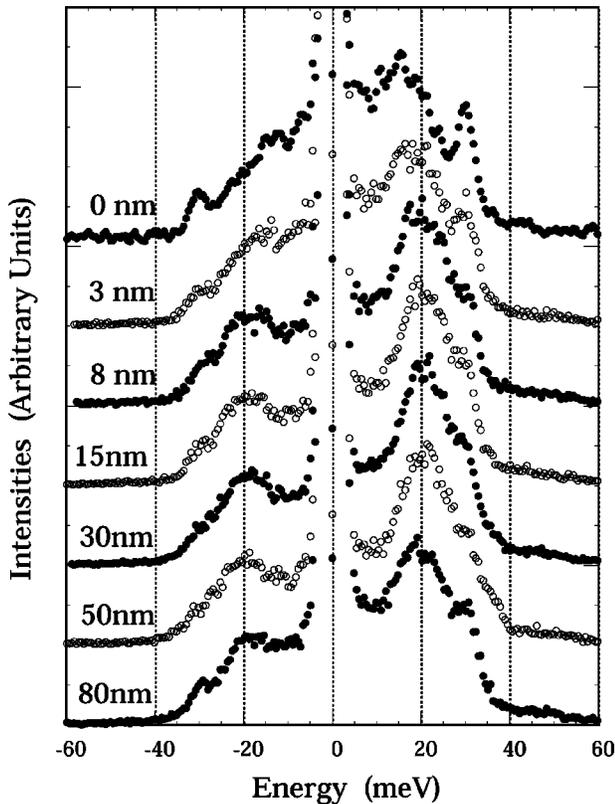
FIG. 1. Nuclear resonant inelastic scattering spectra at room temperature for  $\gamma$ -Fe precipitates with various particle sizes. Here, minus energy indicates the x-ray energy gain process. The data for 0 nm diameter indicate those for the isolated Fe impurities in Cu published by Seto *et al.* (Ref. 5).
