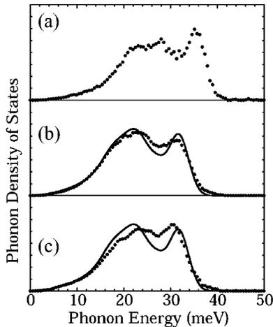
FIG. 3. Experimental phonon density of states at room temperature for (a) bcc-Fe foil, (b) stainless steel (310ss), (c)  $\gamma$ -Fe precipitates in Cu ( $d=80$  nm). Solid lines in (b) and (c) indicate the calculated phonon density of states for  $\text{Fe}_{70}\text{Ni}_{30}$  using the dispersion relation curves determined by neutron inelastic scattering.
