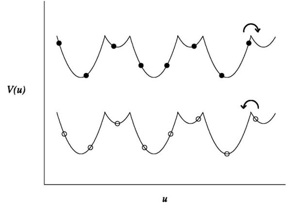
FIG. 3. An example of compatible configurations  $\{u_n\}$  (solid circles) and  $\{u'_n\}$  (open circles), with  $d=2$ ,  $\omega=3/8$ ,  $\beta_1=6/8$ , and  $\beta'_1=5/8$ . By moving the atoms closest to the tip across it (illustrated by the arrows in the figure), corresponding to an elementary phase shift, either of these two configurations is transformed to the other. Compatible configurations are generated by elementary phase shifts.
