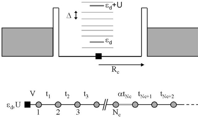
FIG. 1. A sketch of the central grain embedded in a metal (a). Inside the grain the characteristic energy level spacing  $\Delta$  is shown together with the impurity levels at  $\epsilon_d$  and  $\epsilon_d + U$ . In (b) the linear chain obtained after Wilson's canonical transformation.
