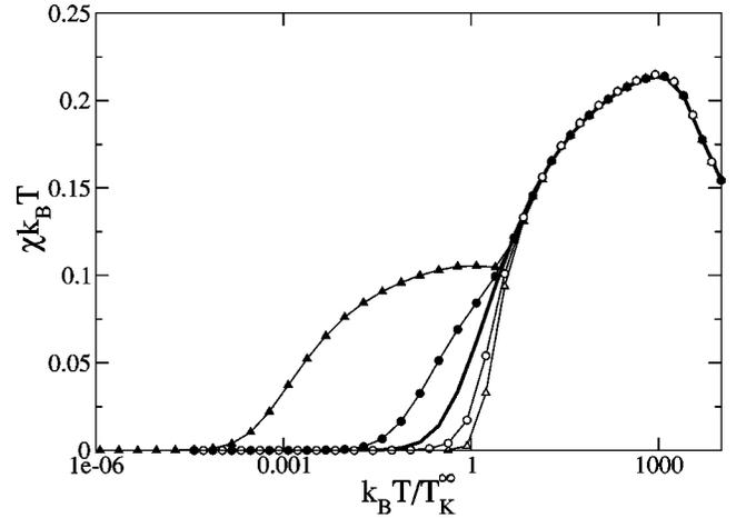
FIG. 3. The magnetic susceptibility  $k_B T \chi$  versus temperature. The thick line corresponds to an impurity in a bulk material ( $\alpha = 1$ ), lines and symbols to a barrier enclosing  $N_c = 19$  and  $20$  shells (open and full symbols, respectively). Triangles (circles) correspond to  $\alpha = 0.35$  ( $0.6$ ). The other parameters are  $\varepsilon_d = -0.5$ ,  $U = 1.0$ , and  $V = 0.2$ .
