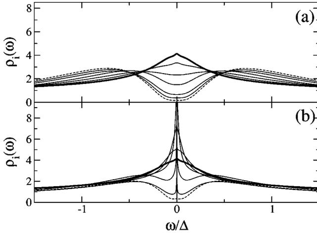
FIG. 6. Impurity spectral density  $\rho_i(\omega, T=0)$  for the at-resonance case with  $N_c=19$  (a) and the off-resonance case with  $N_c=20$  (b) and different values of  $\alpha$ :  $\alpha=0.2$  (dashed line), 0.3, 0.4, 0.6, 0.75, and 0.9 (thick line). ( $\varepsilon_d=-0.5$ ,  $U=1.0$ , and  $V=0.2$ .)
