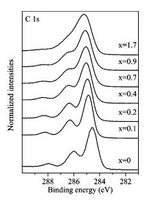
FIG. 5. C 1*s* core-level spectra of CuPc as a function of K intercalation ( $K_x$ CuPc).
