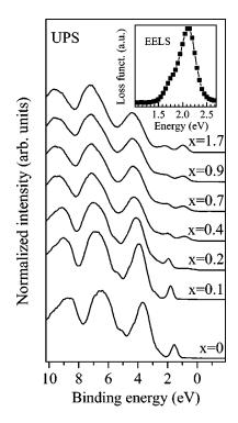
FIG. 2. Valence-band photoemission spectra of CuPc as a function of K intercalation ( $K_x$ CuPc). The inset shows the loss function of pristine CuPc measured using electron energy-loss spectroscopy in transmission of pristine CuPc with an excitation onset of about 1.5 eV which represents the optical energy gap.
