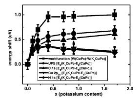
FIG. 3. Energy shift of the C 1*s*, N 1*s*, and Cu  $2p_{3/2}$  core levels; the main features of the valence band (UPS); and the work function upon K intercalation. Since the work function decreases with increasing potassium concentration, we draw the negative shift of the work function to allow a direct comparison of the data.
