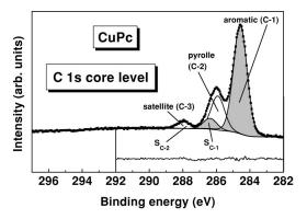
FIG. 4. C 1*s* core-level spectrum of CuPc in the pristine state. One can distinguish between the aromatic carbon and its satellite (gray) and the carbon linked to the nitrogen and its satellite (white). The graph below the spectrum shows the discrepancy between the fit and the spectrum.
