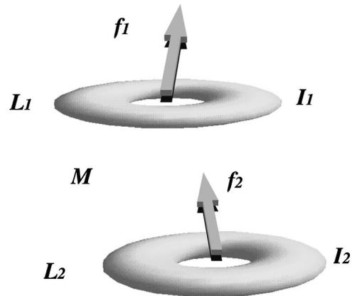
FIG. 1. A drawing of a simple two ring system. The first ring has self-inductance  $L_1$ , and it encloses an external flux  $f_1$ . The second ring has self-inductance  $L_2$  and encloses a flux  $f_2$ . The mutual inductance is  $M$ .
