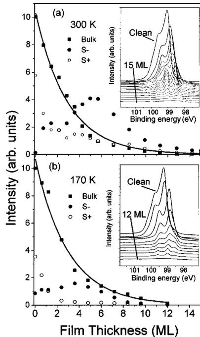
FIG. 1. The components of the Si  $2p$  core-level spectra as a function of film thickness obtained from data recorded at room temperature (a) and at 170 K (b) using a photon energy of 130 eV. The recorded spectra are shown as insets.
