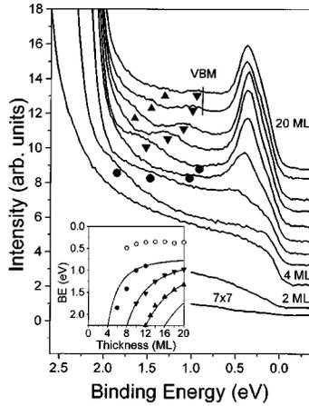
FIG. 3. Cu valence-band spectra recorded with 47-eV photons from a Cu wedge grown at 170 K and annealed to room temperature. The inset shows the thickness dependence of the quantum-well levels along with fits of Eq. (1) to the data. The open symbols show the position of the surface state.
