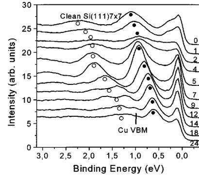
FIG. 4. Valence-band spectra recorded with 47-eV photons from a 10-ML Ag film grown on a Cu wedge (the thickness, given by the numbers on the curves). The symbols in the figure are meant to guide the eye to the shift of peaks with the Cu layer thickness.
