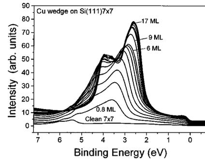
FIG. 2. Cu valence-band spectra recorded with 47-eV photons on a room-temperature-grown Cu wedge.
