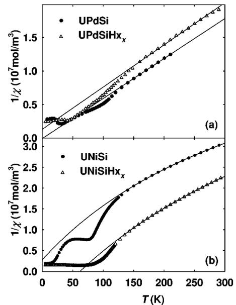
FIG. 5. Inverse susceptibilities of UPdSi-H (a) and UNiSi-H (b) systems. Solid lines indicate the results of the Curie-Weiss fits.
