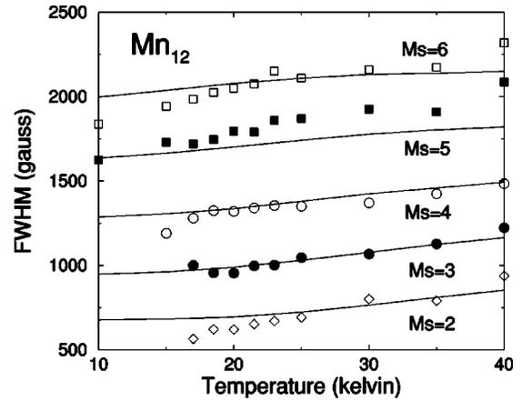
FIG. 8. Calculated (curves) and measured (symbols) FWHM vs temperature at  $\nu=189.123$  GHz for  $\text{Mn}_{12}$ . Here the  $D$  strain ( $\sigma_D \approx 0.018D$ ),  $g$  strain ( $\sigma_g \approx 0.002g$ ), and the dipolar interactions ( $\Gamma \approx 203$   $\text{G}^2$ ) are included in the calculated linewidths.
