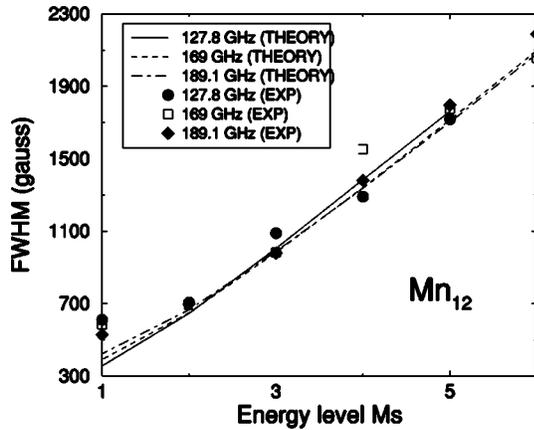
FIG. 9. Calculated (curves) and measured (symbols) FWHM vs energy level  $M_s$  at  $T=20$  K for  $\nu=127.8, 169,$  and  $189.1$  GHz for  $\text{Mn}_{12}$ . Here the values of  $\sigma_D$ ,  $\sigma_g$ , and  $\Gamma$  are the same as those in Fig. 8. Because of a relatively small contribution of the dipolar interaction to the linewidths, the linewidths do not change much with the resonance frequency.
