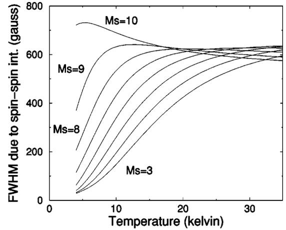
FIG. 5. Calculated FWHM caused by the spin-spin interactions only, shown vs temperature at  $\nu = 116.9$  GHz for  $\text{Fe}_8$ . Here the exchange constant  $J = -7$  G,  $\Gamma \equiv \sum'_{ij} A_{ij}^2/N = 86$  G<sup>2</sup>, and  $\Lambda \equiv \sum'_{ij} J_{ij} A_{ij}/N = -156$  G<sup>2</sup>.
