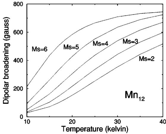
FIG. 7. Calculated FWHM for  $\text{Mn}_{12}$  caused by the dipolar interactions only, shown vs temperature, at  $\nu=189.123$  GHz, with the sum of the squared dipolar interactions  $\Gamma=203$   $\text{G}^2$ . The examined temperature range for  $\text{Mn}_{12}$  is from 10 K to 40 K.
