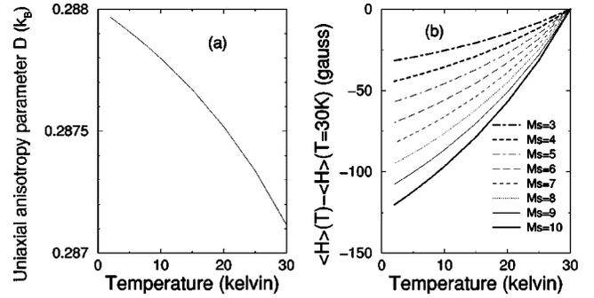
FIG. 1. (a) Hypothetical smooth temperature dependence of the uniaxial anisotropy parameter  $D$  for  $\text{Fe}_8$ . The functional form used here is  $D(T) = -0.710665 + \exp\{-1/[10(50-T)+250]\}$ . (b) The resulting calculated line shifts (the peak position at a given temperature minus the position at  $T=30 \text{ K}$ ) due to this temperature dependence of  $D$ , shown vs temperature at  $\nu=116.9 \text{ GHz}$ .
