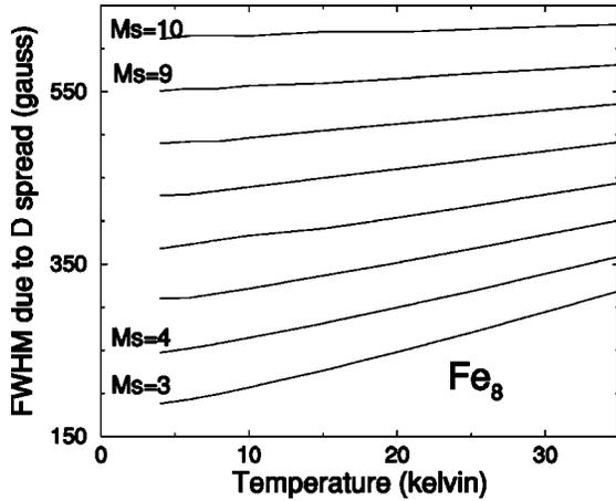
FIG. 4. Calculated full width at half maximum (FWHM), caused by the Gaussian distribution in the uniaxial anisotropy parameter  $D$  only, shown vs temperature from 4 K to 35 K at  $\nu = 116.9$  GHz for  $\text{Fe}_8$ .  $M_s = 10$  indicates the transition from the energy level  $M_s = 10$  to  $M_s = 9$ , etc. The standard deviation of  $D$  is approximately  $0.0064D$ .
