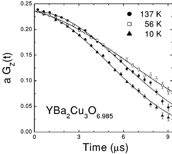
FIG. 1. The time evolution of the muon spin polarization in  $\text{YBa}_2\text{Cu}_3\text{O}_{6.985}$  in zero external field at  $T=10, 56$  and  $137$  K. The signal at  $10$  K relaxes faster than at  $137$  K. At  $56$  K the signal at early times relaxes faster than at  $137$  K, but exhibits a slower relaxation beyond  $5 \mu\text{s}$ .
