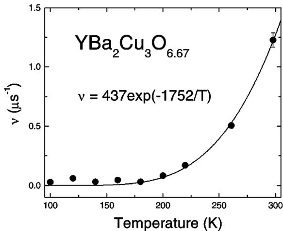
FIG. 4. Plot of the temperature dependence of the  $\mu^+$  hop rate in  $\text{YBa}_2\text{Cu}_3\text{O}_{6.67}$ .
