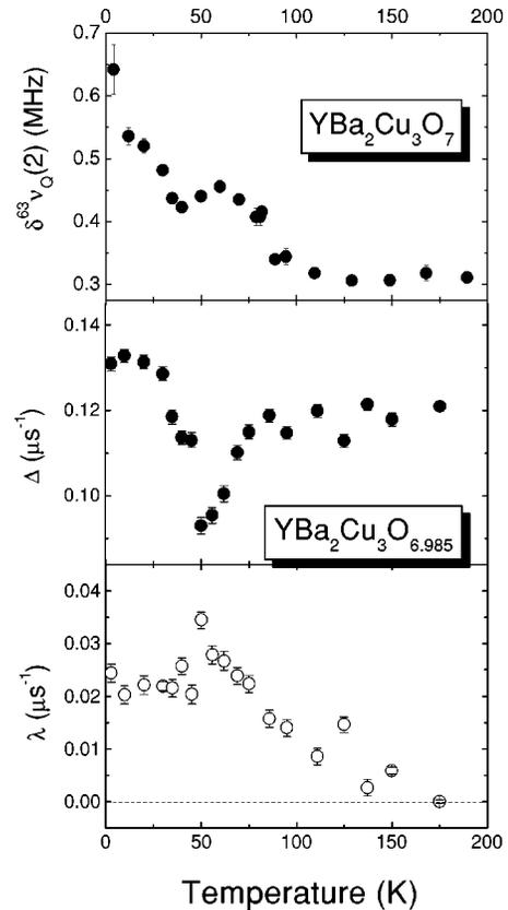
FIG. 5. Temperature dependence of (a)  $\delta^{63}\nu_Q(2)$  in an  $x=1.0$  powdered sample (from Ref. 15) and of (b)  $\Delta$  and (c)  $\lambda$  from fits to the ZF- $\mu$ SR time spectra in  $x=0.985$  crystals to Eq. (2).
