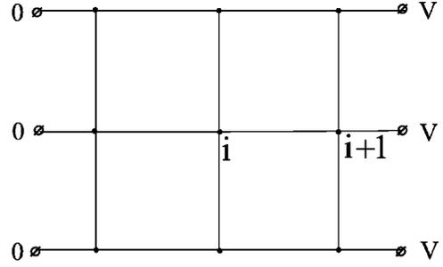
FIG. 4. The net of random resistors. For simplicity, only its 2D projection is presented.
