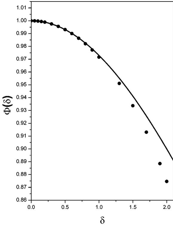
FIG. 5. Factor of disorder. The bold line corresponds to Eq. (21), dots represent average value of  $\Phi$  (over six random realizations of the conductivities) obtained from numerical solution of Eq. (16).
