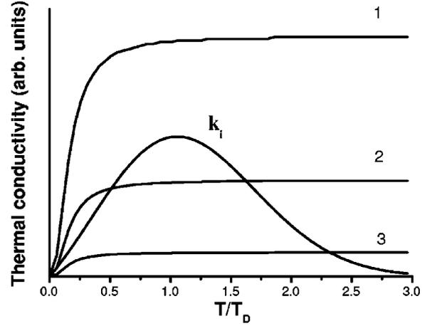
FIG. 7. Temperature dependence of the bulk  $\kappa_i$  and a boundary  $\kappa_{ph}$  parts of TC for the different grain-size nanostructures ( $d_1 > d_2 > d_3$ ).
