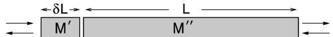
FIG. 1. A small wire with length \delta L , “the building block,” is attached to a long one with length L ( \delta L \ll L ). The total transfer matrix M is given by M = M''M' .
