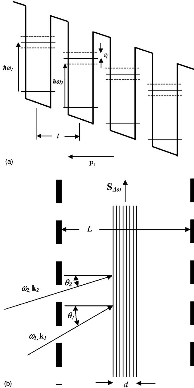
FIG. 1. The energy diagram of BSL under resonant two-frequency pump (a) and a geometry of the THz waveguide with excitation scheme (b).
