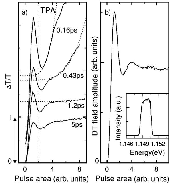
FIG. 2. (a) Time-integrated differential transmission probe intensity versus pump-pulse area measured for different pulse durations at 1.16-eV spectral position and 1-mA injection current. Curves are vertically displaced for clarity. The vertical dashed line is a guide for the eyes. Dotted lines show the effect of two-photon absorption (TPA). (b) Differential transmission probe field amplitude for a spectrally square-shaped pulse. The pulse spectrum is shown in the inset.
