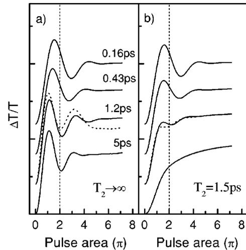
FIG. 4. Differential transmission intensity calculated for different pulse durations, as indicated, for an infinitely long dephasing time (a) and 1.5-ps dephasing time (b), vertically displaced for clarity. Dotted lines are calculations for a spectrally square-shaped pulse of  $\sim 1$ -ps duration. The  $2\pi$  pulse area is marked with a dashed line, for reference.
