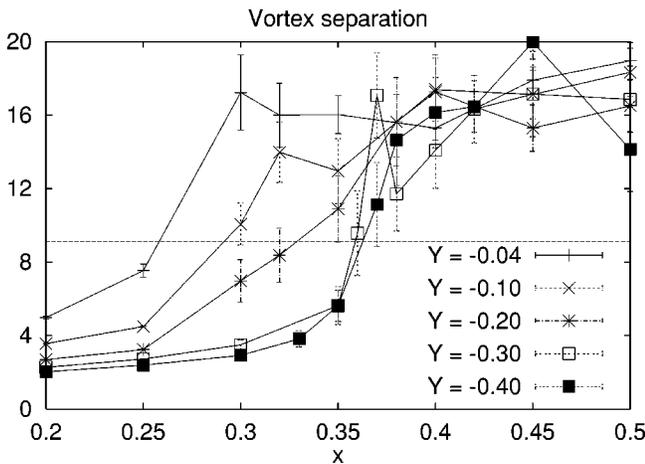
FIG. 5. The ensemble-averaged distance between a pair of vortices,  $\langle d \rangle$ , as a function of the square of the Ginzburg-Landau parameter  $x = \kappa^2$ , for various values of the temperaturelike variable  $y$ . The horizontal line is at  $d_0/2$ . Increasing  $y$  amounts to increasing the temperature.
