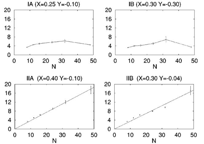
FIG. 1. The ensemble-averaged separation  $\langle d \rangle$  between the two vortices, as a function of system size. The two upper figures are indicative of type-I behavior, whereas the two lower ones indicate type-II behavior.
