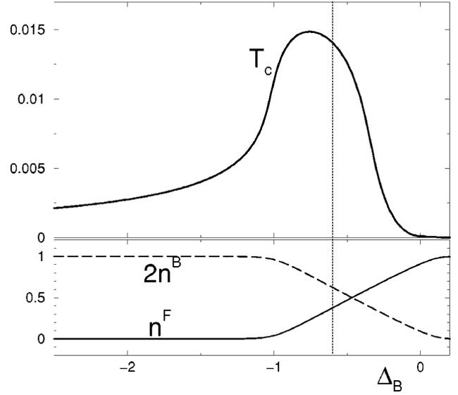
FIG. 1. Variation of  $T_c$  with respect to the boson energy  $\Delta_B$  for a clean system with  $n_{tot} = 1$ . The bottom panel illustrates the concentrations of fermions ( $n^F$ ) and bosons ( $n^B$ ) at  $T = T_c$ . Note the three distinct regimes: predominantly local pairs  $2n^B \sim n_{tot}$ , coexisting pairs and fermions  $n^F \sim 2n^B$ , and predominantly fermions  $n^F \sim n_{tot}$  (the so-called BCS limit).
