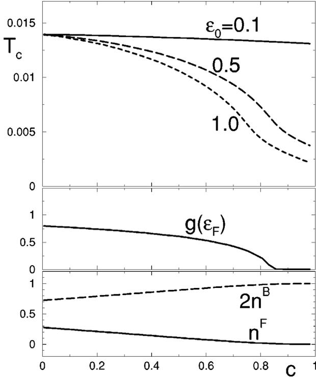
FIG. 2. Transition temperature  $T_c$  as a function of concentration  $c$  of scattering centers with various positive values of  $\varepsilon_0$  (top panel). Density of states at the Fermi energy  $g(\varepsilon_F)$  (middle panel) and relative occupations by bosons and fermions (bottom panel) for  $\varepsilon_0=0.5$  at  $T=T_c$ .
