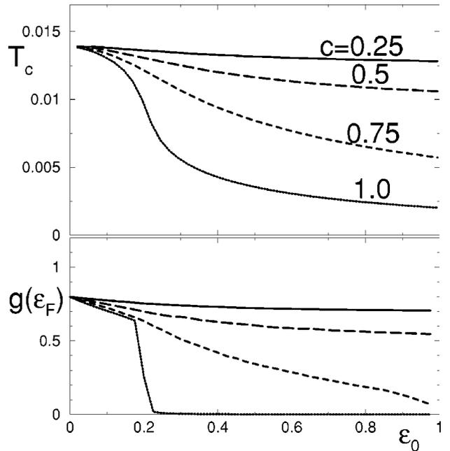
FIG. 4. Transition temperature  $T_c$  as a function of the energy  $\varepsilon_0$  of the scattering centers whose concentration is  $c$  (top). Density of states  $g(\varepsilon_F)$  for each of the concentrations  $c$  (bottom panel). For  $c=1$  and  $\varepsilon_0 \geq 0.2$  the Fermi energy goes below the fermion band. The system is then strictly in the LP limit of the BF model.
