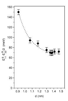
FIG. 6. The difference between the energy of the lowest lying interband transition  $(E_{11}^S)$  and half of that of the second transition  $(E_{22}^S)$  in SWCNT's with different mean diameters as a function of the SWCNT mean diameter. Deviation from the value 0.5 is an indication of Coulomb interaction effects, which most strongly affect the energy position of  $E_{11}^S$  (for details see text).
