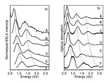
FIG. 4. (a) Loss function in the region of the low-energy interband transitions for SWCNT's with different mean diameters recorded with  $q = 0.1 \text{ Å}^{-1}$ . (b) Optical absorption spectra (after background subtraction) from SWCNT with mean diameters as indicated.
