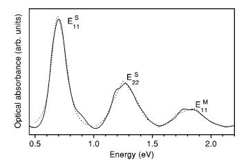
FIG. 7. Simulation of the first three optical absorption peaks of sample B with d=1.37 nm upon the basis of tight binding calculations. Nanotubes of all chiralities are included. The solid line is the measured spectrum (with background subtracted); the dotted line represents the results of the simulation.
