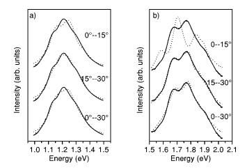
FIG. 8. The tight-binding-based fitting of the (a)  $E_{22}^S$  and (b)  $E_{11}^M$  optical absorption features of sample A with d = 1.46 nm. The solid line is the measured data (background subtracted), and the dashed lines are the simulations using a SWCNT chiral angle distribution as indicated. 30° stands for armchair, 0° for a zigzag nanotube.
