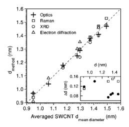
FIG. 9. Correlation plot of the SWCNT's mean diameters  $d_{\text{method}}$  determined by different bulk sensitive methods. The horizontal axis is the SWCNT's  $d_{\text{mean}}$  averaged over all methods. The Raman and x-ray results are from Ref. 12. The inset shows the plot of the diameter distribution  $\Delta d$  versus different mean diameters (full solid), where the open square presents the data obtained from Raman spectroscopy in Ref. 12
