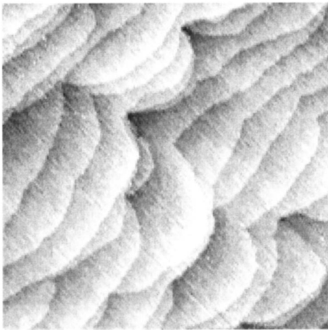
FIG. 4. Scanning tunneling micrograph of the InP (001) surface after a 20-min H_2 anneal in the MOVPE reactor at 500 °C (image size = 0.15 \times 0.15 \mu m^2 ).
