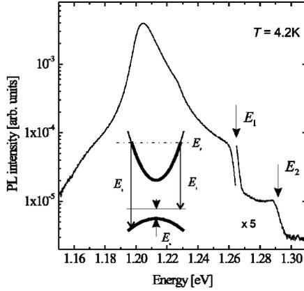
FIG. 1. Photoluminescence spectrum of the modulation doped GaAs/InGaAs/AlGaAs QW with a high density of the 2DEG measured at  $T=4.2$  K in zero magnetic field. Two PL cutoffs at the energies  $E_1$  and  $E_2$  (see long arrows) are shown. Recombination scheme for the PL observed at  $E_1$  and  $E_2$  is shown in the inset.
