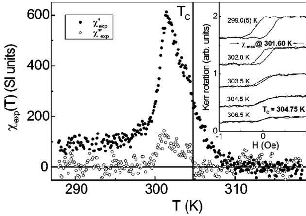
FIG. 1. Real  $\chi'_{exp}(T)$  (solid circles) and imaginary part  $\chi''_{exp}(T)$  (open circles) of the experimental susceptibility  $\chi_{exp}(T)$  at  $H_0 = 17$  mOe. The temperature at the onset of  $\chi''_{exp}(T)$  marks  $T_C = 304.75$  K (vertical solid line). Inset: Temperature-dependent dc-MOKE measurements around  $T_{max} = 301.6$  K of  $\chi'_{exp}(T)$ .
