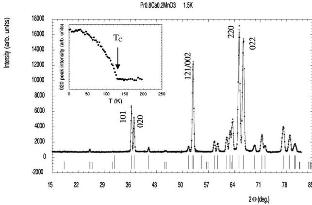
FIG. 1. 1.5-K neutron diffraction patterns: continuous line for calculated plot, stars for experimental data; the upper Bragg strikes correspond to the  $Pnma$  crystallographic structure and the lower one to the magnetic phase. The main indexations are also given. Inset: 020 FM peak intensity vs temperature.
