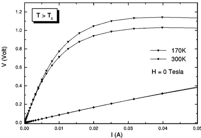
FIG. 4.  $V$ - $I$  characteristics under zero field for temperatures above  $T_c$  (170 and 300 K).
