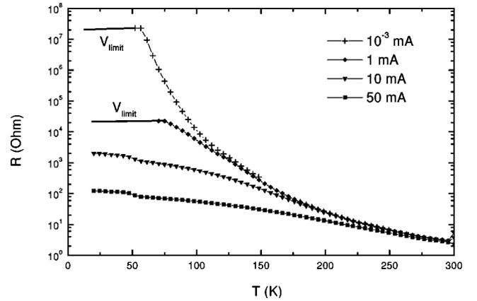
FIG. 2. Temperature dependence of resistance for a  $\text{Pr}_{0.8}\text{Ca}_{0.2}\text{MnO}_3$  crystal with various bias currents.
