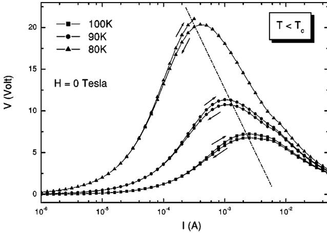
FIG. 3.  $V$ - $I$  characteristics under zero field for temperatures below  $T_c$  (80, 90, and 100 K).
