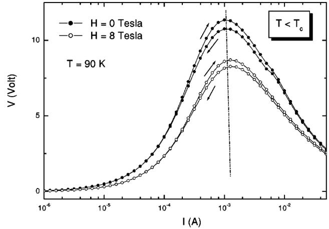
FIG. 5.  $V$ - $I$  characteristics for  $T = 90$  K under 0 and 8 T.
