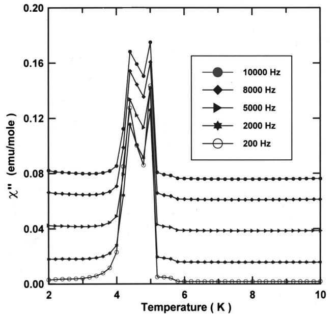
FIG. 6. The temperature dependence of the imaginary component of ac susceptibilities  $\chi''(T)$  for  $\text{CeNi}_2\text{Sn}_2$  in an ac field of 0.0001 T at 200, 2000, 5000, 8000, and 10 000 Hz.
