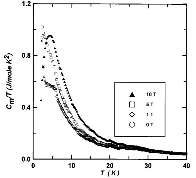
FIG. 10. The magnetic molar specific heat divided by temperature  $C_m/T$  versus temperature in 0, 1, 5, and 10 T for  $\text{CeNi}_2\text{Sn}_2$ . The magnetic specific-heat  $C_m$  is defined as  $C_m = C(\text{CeNi}_2\text{Sn}_2) - C(\text{LaNi}_2\text{Sn}_2)$ .
