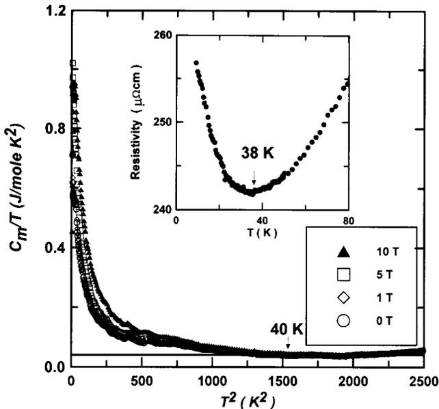
FIG. 11.  $C_m/T$  vs  $T^2$  in 0, 1, 5, and 10 T for CeNi<sub>2</sub>Sn<sub>2</sub>. The inset is the temperature dependence of resistivity for CeNi<sub>2</sub>Sn<sub>2</sub> between 10 and 80 K.
