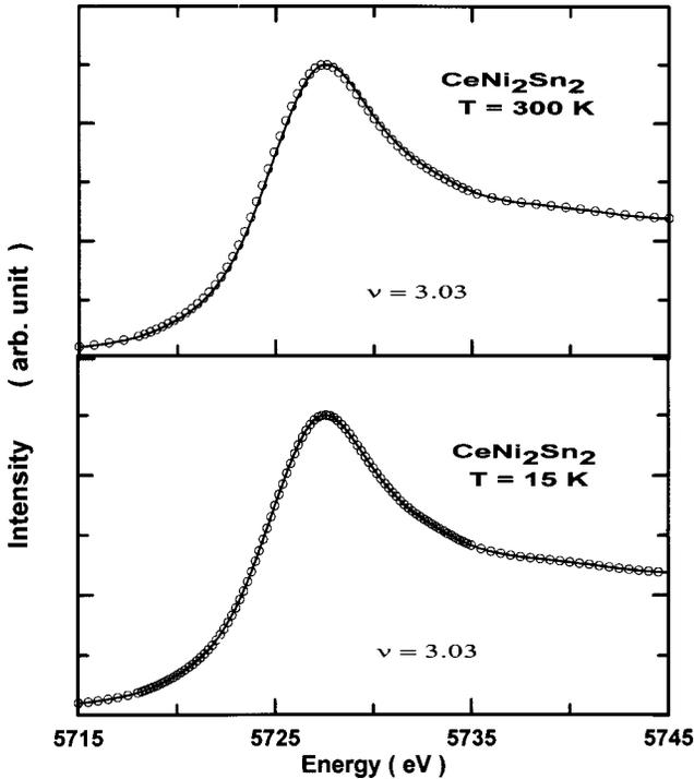
FIG. 12. The Ce  $L_{III}$ -edge spectra of  $CeNi_2Sn_2$  at 300 and 15 K. The solid lines are fitting curves.
