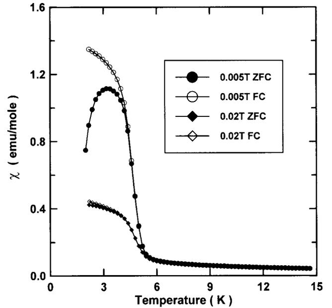
FIG. 3. The temperature dependence of the zero-field-cooled molar susceptibility  $\chi_{ZFC}(T)$  and field-cooled molar susceptibility  $\chi_{FC}(T)$  for  $\text{CeNi}_2\text{Sn}_2$  at 0.005 and 0.02 T.
