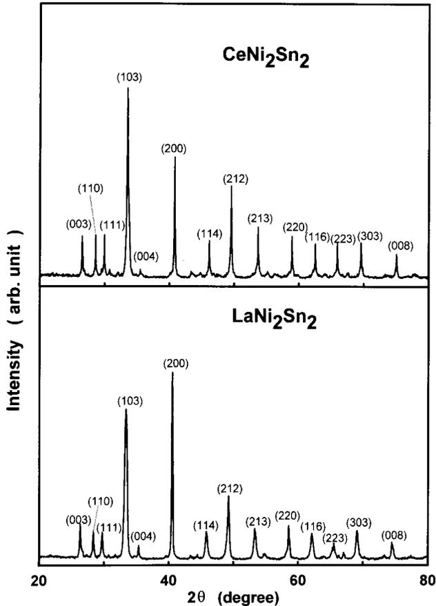
FIG. 1. The x-ray-diffraction patterns of  $\text{CeNi}_2\text{Sn}_2$  and  $\text{LaNi}_2\text{Sn}_2$ .
