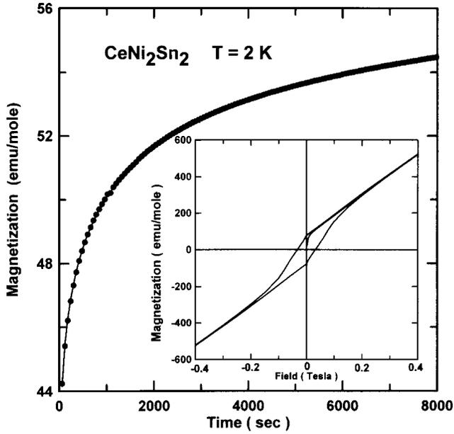
FIG. 4. The time dependence of zero-field cooled magnetization  $M_{\text{ZFC}}(t)$  for  $\text{CeNi}_2\text{Sn}_2$  at 2 K in a 0.005-T field. The solid line is the fitting curve of stretched exponential function:  $M_{\text{ZFC}}(t) = M_0 - M' \exp[-(t/\tau)^{1-n}]$  with  $\tau = 917$  s. The inset is the field dependence of magnetization  $M(H)$  at 2 K.
