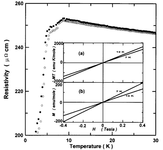
FIG. 8. The temperature dependence of zero-field-cooled electrical resistivity  $\rho_{ZFC}(T)$  (●) and field-cooled resistivity  $\rho_{FC}(T)$  (○) in a 0.0050-T magnetic field between 2 and 30 K.
