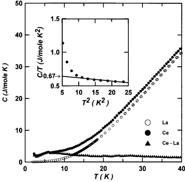
FIG. 9. The temperature dependence of specific heat  $C(T)$  for  $\text{CeNi}_2\text{Sn}_2$  (●) and  $\text{LaNi}_2\text{Sn}_2$  (○). The magnetic specific heat  $C_m$  (▲) was defined as  $C_m = C(\text{CeNi}_2\text{Sn}_2) - C(\text{LaNi}_2\text{Sn}_2)$ . The inset is  $C/T$  versus  $T^2$  between 2 and 5 K.
