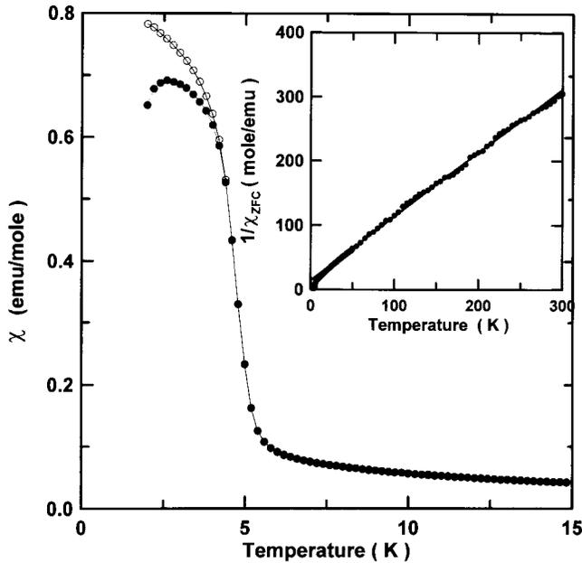
FIG. 2. The temperature dependence of the zero-field-cooled molar susceptibility  $\chi_{ZFC}(T)$  (●) and field-cooled molar susceptibility  $\chi_{FC}(T)$  (○) for  $\text{CeNi}_2\text{Sn}_2$  at a 0.01 T magnetic field. The inset is the temperature dependence  $1/\chi_{ZFC}(T)$  for  $\text{CeNi}_2\text{Sn}_2$  at a 0.01-T magnetic field.
