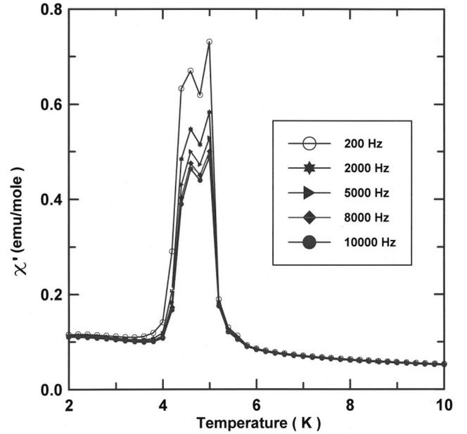
FIG. 5. The temperature dependence of the real component of ac susceptibilities  $\chi'(T)$  for  $\text{CeNi}_2\text{Sn}_2$  in an ac field of 0.0001 T at 200, 2000, 5000, 8000, and 10 000 Hz.
