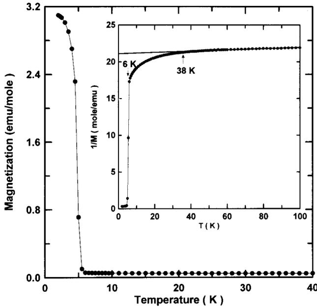
FIG. 7. The temperature dependence of magnetization  $M(T)$  without any applied field. The inset is the inverse of magnetization  $M^{-1}(T)$  versus temperature.
