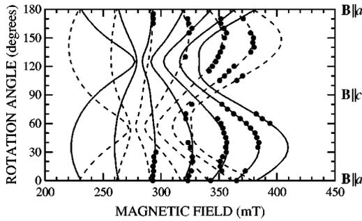
FIG. 3. Photoinduced STH signals (closed circles) vs rotation angle measured at 8 K. Microwave frequency is  $9.383(\pm 0.002)$  GHz. Magnetic-field vector  $\mathbf{B}$  is in the  $ac$  plane and the rotation axis is the  $b$  axis. Solid and dashed lines: fitting lines derived from the spin Hamiltonian described in Sec. IV B.
