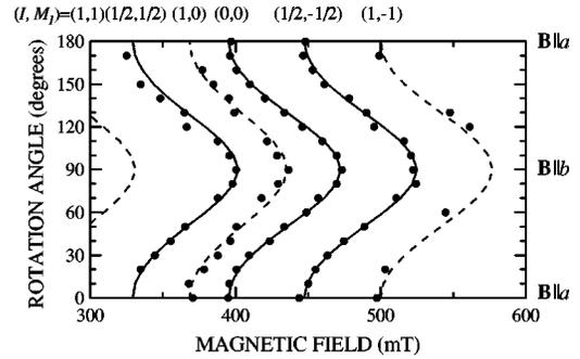
FIG. 2. Photoinduced STEL signals (closed circles) vs rotation angle measured at 8 K. Microwave frequency is 9.371( $\pm 0.001$ ) GHz. Magnetic-field vector  $\mathbf{B}$  is in the  $ab$  plane and the rotation axis is the  $c$  axis.  $(I, M_I)$ : the total nuclear spin of the STEL centers and the magnetic quantum number. Solid and dashed lines: fitting lines derived from the spin Hamiltonian described in Sec. IV A.
