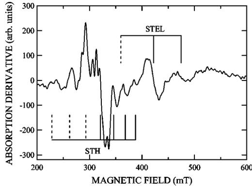
FIG. 1. Typical ESR spectrum measured at 5 K after photoirradiation at 5 K. Magnetic-field vector is in the  $ac$  plane and the direction corresponds to  $65^\circ$  in Fig. 3 below. Microwave frequency is 9.385 GHz. STEL and STH are described in Sec. III A. Solid lines indicate the prominent ESR positions. Dashed lines correspond to the ESR positions calculated from the spin Hamiltonian in Sec. IV.
