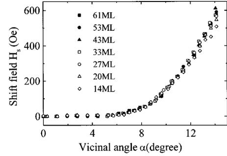
FIG. 4. Shift field  $H_S$  vs the vicinal angle  $\alpha$  with several different Fe film thicknesses.
