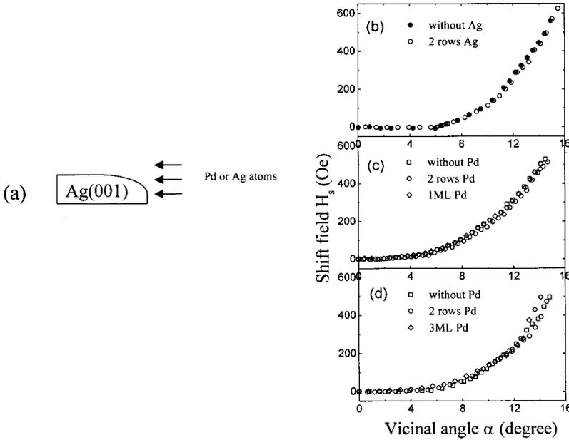
FIG. 5. (a) Schematic drawing of the side-growth geometry. The shift field  $H_s$  vs the vicinal angle  $\alpha$  of (b) 15 ML Fe prior to and after Ag step decoration on the Fe film, (c) 30 ML Fe prior to and after Pd decoration on the Fe film, and (d) 27 ML Fe prior to and after Pd decoration on the Ag substrate.
