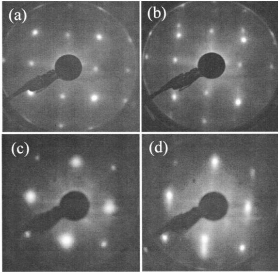
FIG. 1. LEED patterns from (a) flat Ag(001), (b) stepped Ag(001) with  $\sim 11^\circ$  vicinal angle, (c) 25 ML Fe grown on flat Ag(001), and (d) 25 ML Fe grown on stepped Ag(001) with  $\sim 11^\circ$  vicinal angle. The electron energy is  $\sim 137$  eV in (a) and (b) and  $\sim 94$  eV in (c) and (d).
