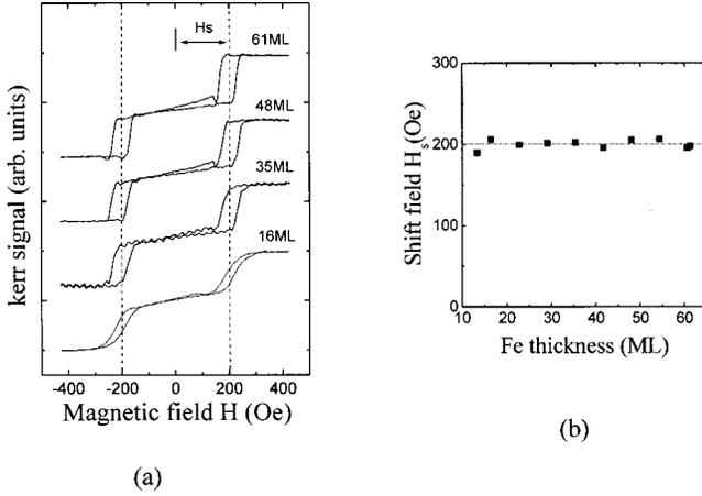
FIG. 3. (a) Hard-axis hysteresis loops of Fe films grown on a curved Ag(001) substrate at a vicinal angle of  $10.5^\circ$ . The shift field  $H_S$  (dashed line) measures the strength of the step-induced magnetic anisotropy. (b) The shift field  $H_S$  vs the Fe film thickness.
