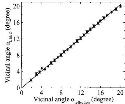
FIG. 2. Relationship between the vicinal angle obtained from Ag double LEED spots and the vicinal angle obtained from a laser beam reflection measurement. The solid line is a linear fit to the data with a slope of 1.02.
