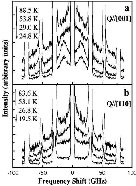
FIG. 1. Temperature dependence of the light-scattering spectra of STO18 above 20 K taken with (a)  $Q\parallel[001]$  and (b)  $Q\parallel[110]$ , where  $Q$  is the scattering vector.
