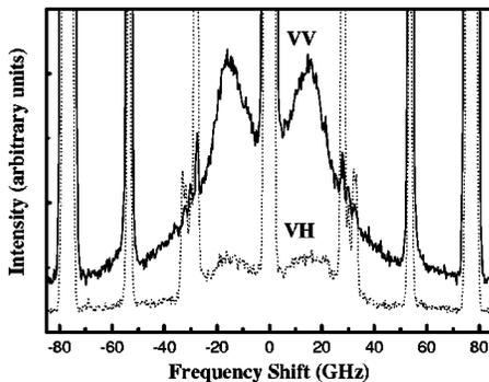
FIG. 5. Polarization dependence of the light-scattering spectra of the broad doublet in STO18. VV indicates vertical polarization of both incident and scattered light, VH indicates vertical polarization of incident light and horizontal polarization of scattered light with respect to the scattering plane.
