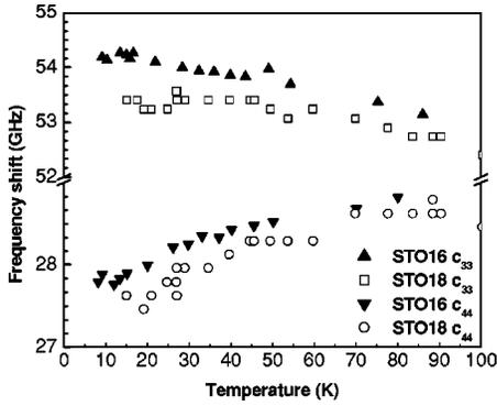
FIG. 4. Temperature dependence of the frequency shifts of the  $c_{33}$  and  $c_{44}$  acoustic modes for STO18 and STO16.
