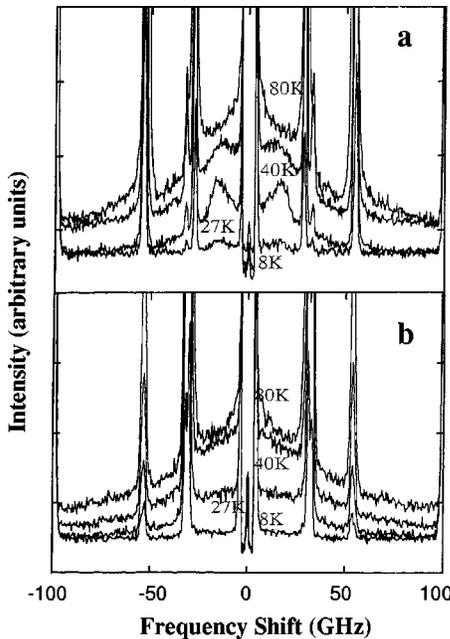
FIG. 2. Temperature dependence of the light-scattering spectra of STO16 taken with (a)  $Q\parallel[001]$  and (b)  $Q\parallel[110]$ .
