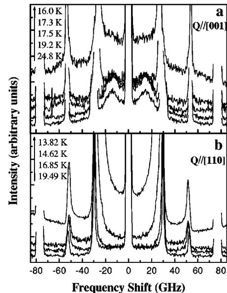
FIG. 6. Temperature dependence of the light-scattering spectra of STO18 near the ferroelectric phase-transition point  $T_C$  with (a)  $Q\parallel[001]$  and (b)  $Q\parallel[110]$ .
