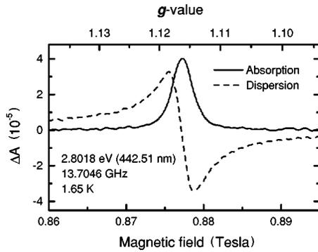
FIG. 2. The absorption and dispersion components of the CR-ESR spectrum from a ZnSe epitaxial layer. The incident microwave and laser powers were, respectively, 100 mW and 40 mW.
