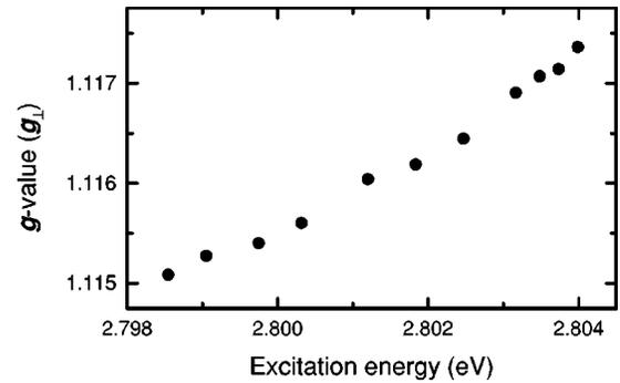
FIG. 3. The dependence of the measured value of  $g_{\perp}$  on the laser energy.
