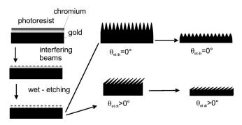
FIG. 10. Sketch of the different steps for the preparation of the deep gold gratings.
