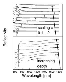
FIG. 16. Modeled (top) and measured (bottom) wavelength-dependent reflectivity ( $\theta=4^\circ$ ,  $\psi=90^\circ$ ) from a grating etched under  $\theta_{etch}=30^\circ$  for different grating amplitudes. The position of the ME<sub>1</sub> resonance is indicated by open circles in the calculated data. The thicker line corresponds to the grating shape as determined by electron microscopy.
