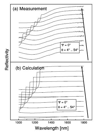
FIG. 18. Modeled (top) and measured (bottom) wavelength-dependent reflectivity of the grating that was etched at  $\theta_{etch}$ = 40° as a function of wavelength. Different polar angles  $\theta$  are chosen for  $\psi$ =0° (classical mount). The straight horizontal line in (b) is added to the graph as a guide to the eye to see the reflectivity minimum.
