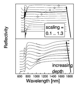
FIG. 17. Modeled (top) and measured (bottom) wavelength-dependent reflectivity ( $\theta=4^{\circ}$ ,  $\psi=90^{\circ}$ ) from a grating etched under  $\theta_{etch}=40^{\circ}$  for different grating amplitudes. A weak resonance is marked by open circles where it is hard to see. The thicker line corresponds to the grating shape as determined by electron microscopy.
