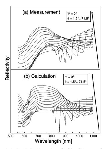
FIG. 21. Wavelength-dependent reflectivity of the symmetric grating ( $\Lambda$  = 654.5 nm) in the classical mount ( $\psi$ =0°) for polar angles ( $\theta$ ) between 1.5° and 71.5° as obtained from measurement (top) and theory (bottom).
