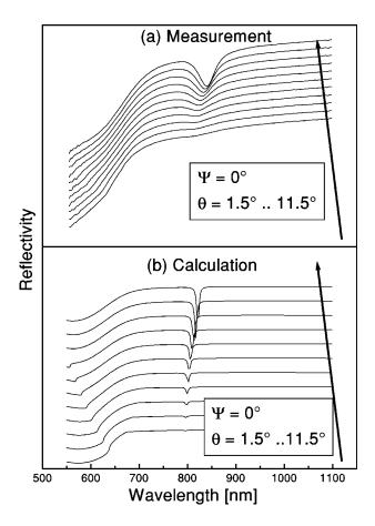
FIG. 20. Measured (top) and modeled (bottom) wavelength-dependent reflectivity (TM polarization) of the symmetric grating ( $\Lambda = 654.5$  nm) for varying polar angle  $\theta$  in the classical mount ( $\psi = 0^{\circ}$ ).
