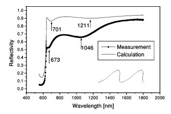
FIG. 15. Wavelength-dependent reflectivity ( $\theta = 4^{\circ}$ ,  $\psi = 90^{\circ}$ ) of the grating etched at  $\theta_{etch} = 30^{\circ}$  as determined from a measurement compared to theory. The surface profile as determined by electron microscopy is shown in the graph.
