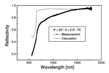
FIG. 19. Wavelength-dependent reflectivity ( $\theta$ =4°,  $\psi$ =90°) of a symmetric grating ( $\Lambda$ =654.5 nm). The dots mark measured points and the straight line is based on theory.
