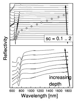
FIG. 14. Modeled (top) and measured (bottom) wavelength-dependent reflectivity ( $\theta=4^{\circ}$ ,  $\psi=90^{\circ}$ ) from a grating etched under  $\theta_{etch}=10^{\circ}$  with scaling factors applied to the grating profile underlying the calculation, which vary between 0.1 and 2. The position of the ME<sub>1</sub> resonance is indicated by open circles. The thicker line corresponds to the grating shape as determined by electron microscopy.
