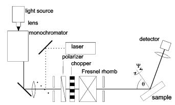
FIG. 12. Sketch of the optical setup for reflectivity measurements.
