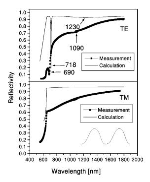
FIG. 13. Wavelength-dependent reflectivity ( $\theta$ =4°,  $\psi$ =90°) from a grating etched under  $\theta_{etch}$ =10° for TM and TE polarization. The theoretical curve is based on the grating profile that is shown in the inset.
