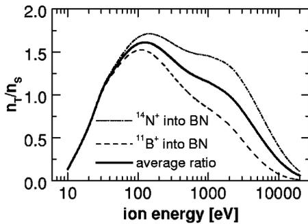
FIG. 1. Parameter  $n_T/n_S$  calculated for  $^{11}\text{B}$  and  $^{14}\text{N}$  ion deposition into boron nitride (from Ref. 8).
