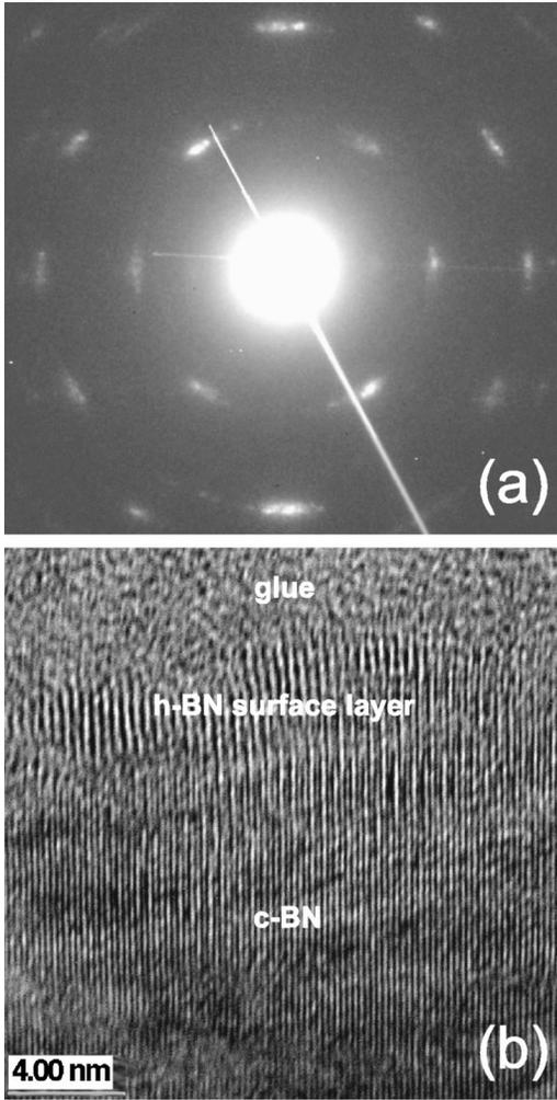
FIG. 3. (a) Electron diffraction image of the top half of the 5 keV BN film showing the typical  $c$ -BN pattern. (b) TEM cross-sectional view of the surface region of the 5 keV BN film, showing the  $c$ -BN planes extending up to the film surface covered only by a thin  $sp^2$  surface layer.
