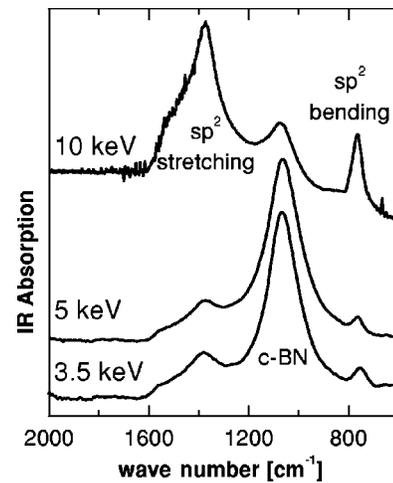
FIG. 2. FTIR spectra of BN films grown on *c*-BN with ion energies of 3.5, 5, and 10 keV, respectively. The stretching and bending absorption peaks at  $1380$  and  $750 \text{ cm}^{-1}$ , respectively, are typical for  $sp^2$ -bonded BN. The absorption peak around  $1070 \text{ cm}^{-1}$  is due to the characteristic *c*-BN reststrahlen band.
