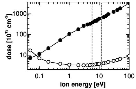
FIG. 4. Open circles: Required dose to accumulate a defect concentration of 1 dpa within the mean ion range by ion bombardment of a  $3.5 \text{ g/cm}^3$  BN target with B and N ions. Solid circles: Required dose to grow a BN layer with thickness equal to the mean ion range with sputter losses included. The doses were calculated with TRIM (Ref. 21). The dashed lines indicate the  $c$ -BN to  $sp^2$ -bonded BN transition region.
